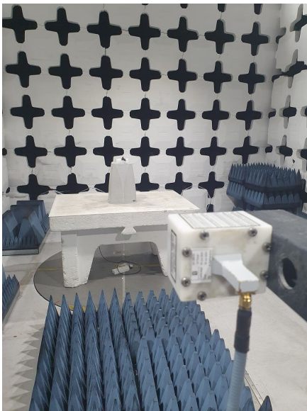
Radiated emissions test set up above 18GHz.
