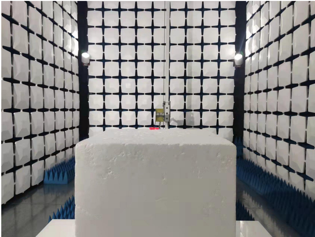
Above 1GHz for radiated emission test setup
