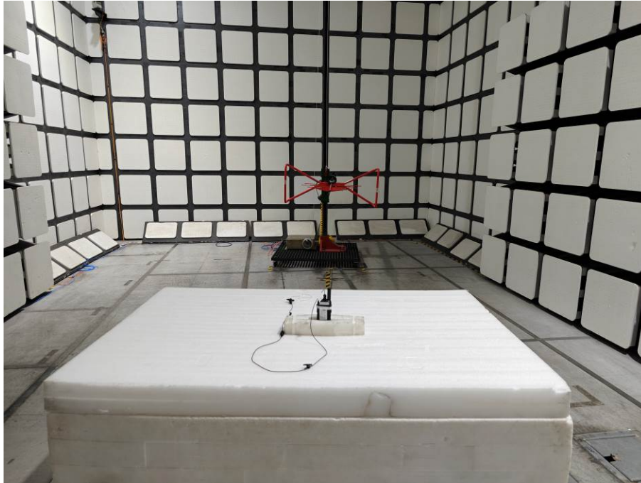
Radiated Emissions View (Below 1 GHz)
