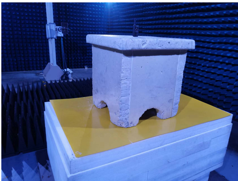
Photo of Radiated Emission Measurement (Above 1G)
