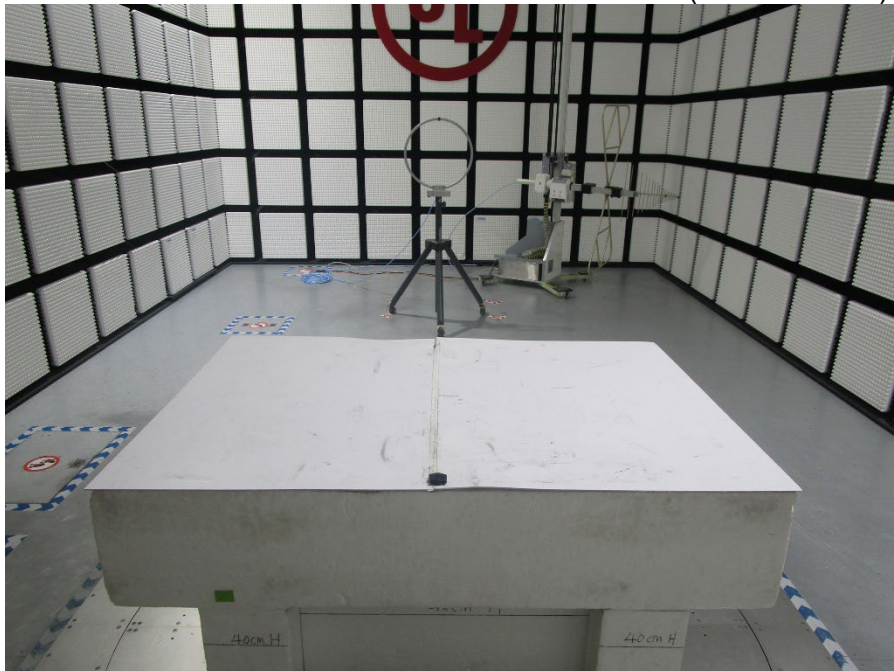
RADIATED EMISSIONS MEASUREMENT SETUP (Below 30MHz)
