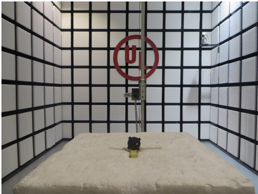
RADIATED EMISSIONS MEASUREMENT SETUP (Above 1G– Y axis)
