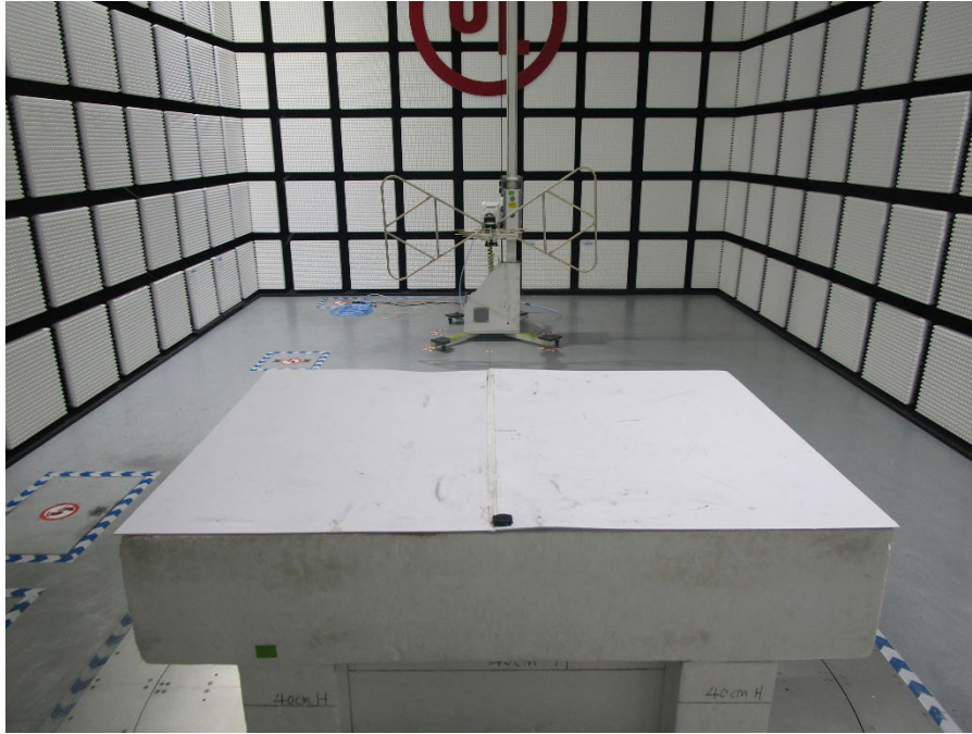
RADIATED EMISSIONS MEASUREMENT SETUP (Below 30MHz)
