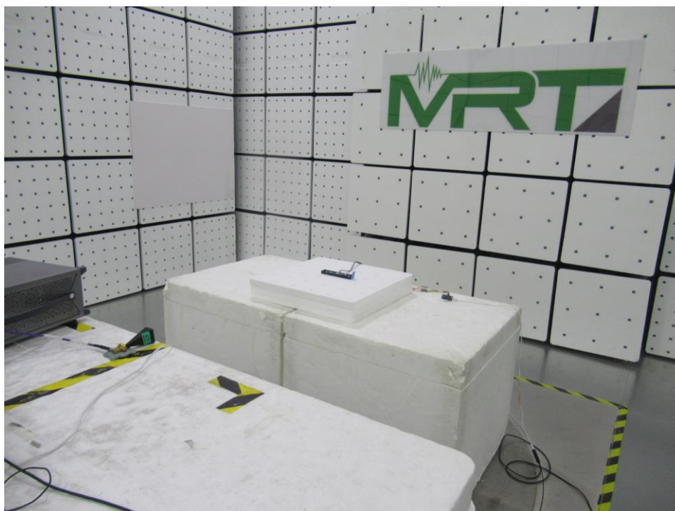
Photograph 4: Set-up photo for Radiated Spurious Emission, 40GHz - 50GHz
