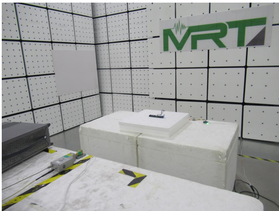
Photograph 6: Set-up photo for Radiated Spurious Emission, 75GHz - 100GHz
