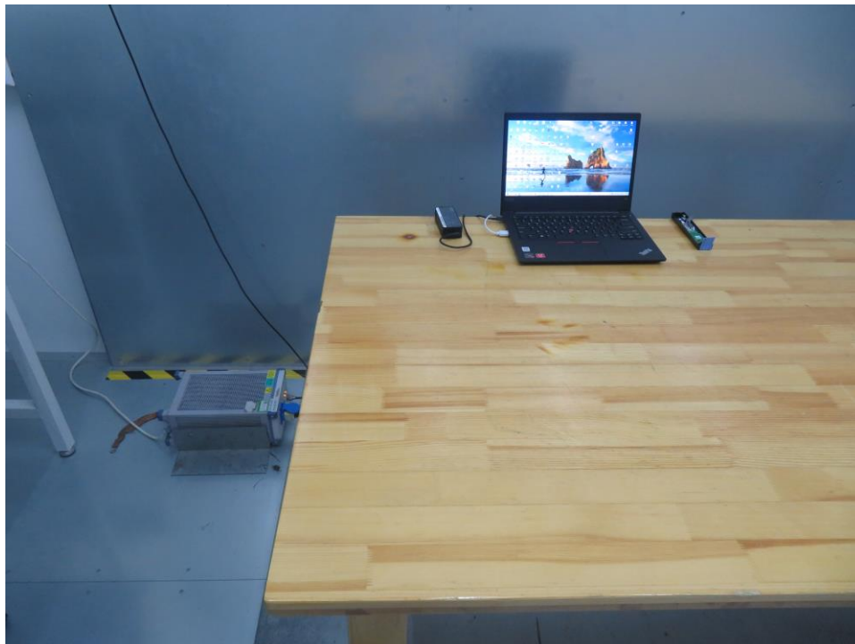
Photograph 7: Set-up for Conducted Emission on AC Mains
