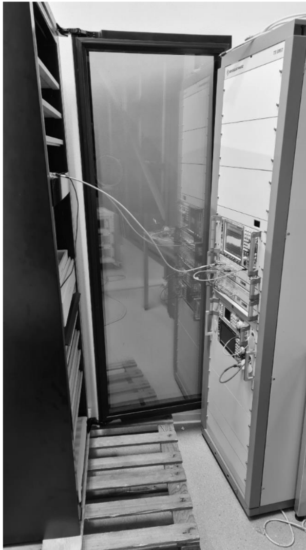
Figure 5: Conducted measurements test setup
