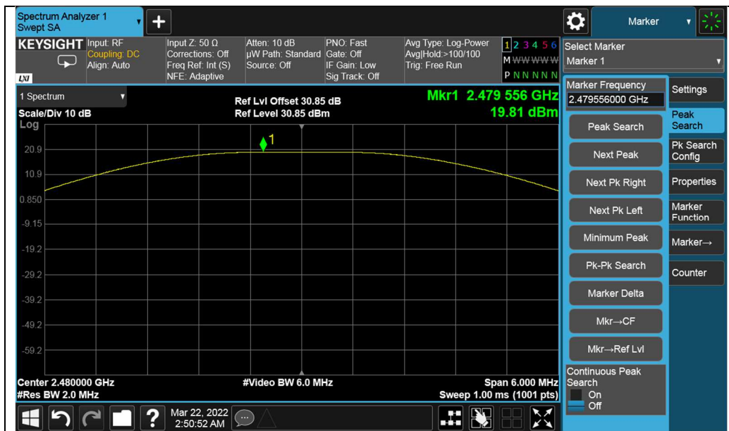
Conducted Output Power Ch. 26
