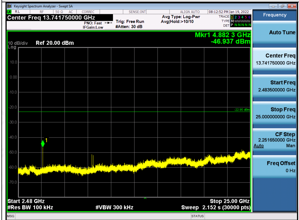
Test_Graph_BR_ANT1_2441_1Mbps_Higher Band Emissions
