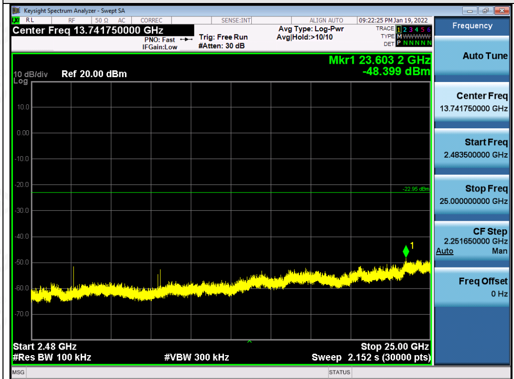
Test_Graph_EDR_ANT1_2441_3Mbps_Higher Band Emissions
