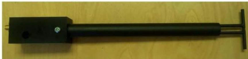
Figure 1 – MVG COMOSAR Validation Dipole
