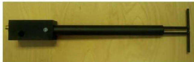
Figure 1 – MVG COMOSAR Validation Dipole
