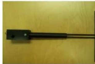
Figure 1 – MVG COMOSAR Validation Dipole
