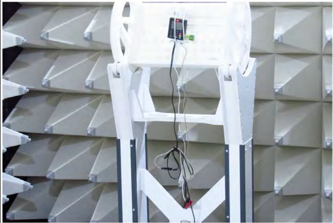
Setup EUT view above 1GHz
