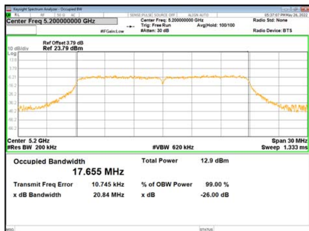
(802.11ac20) plot on channel 48
