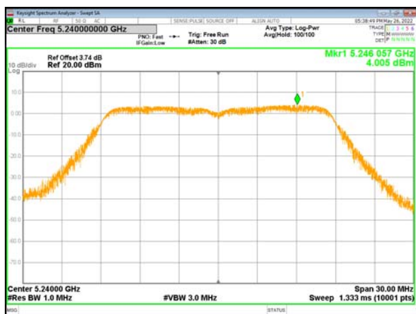
(802.11ac20) PSD plot on channel 48
