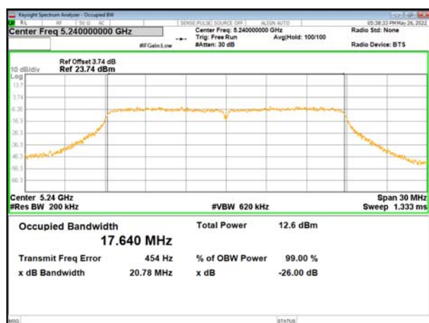
(802.11ac20) plot on channel 48
