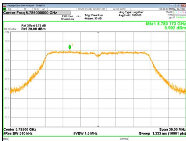
(802.11ac20) PSD plot on channel 165
