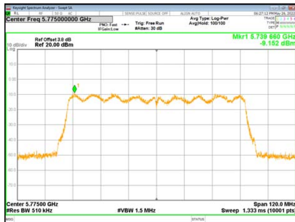
(802.11ac80) PSD plot on channel 155
