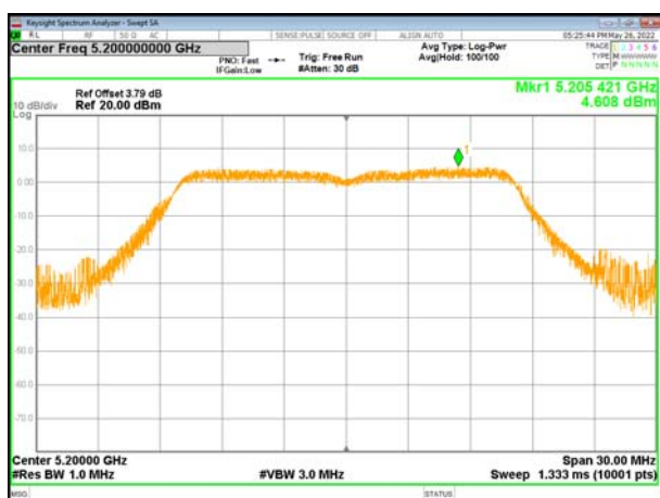
(802.11a) PSD plot on channel 40
