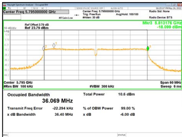
(802.11 ac40) plot on channel 159
