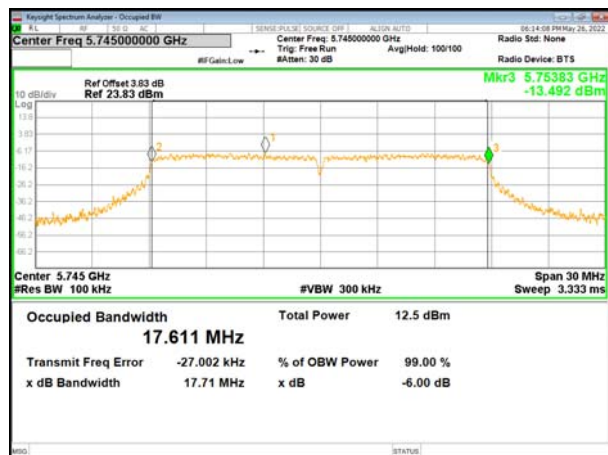
(802.11ac20) plot on channel 157
