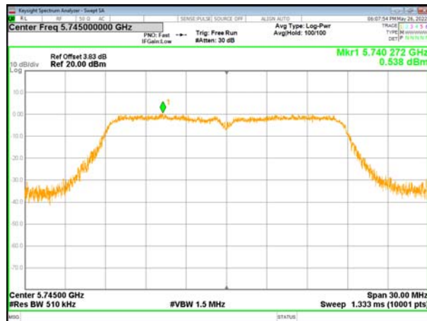
(802.11n20) PSD plot on channel 157
