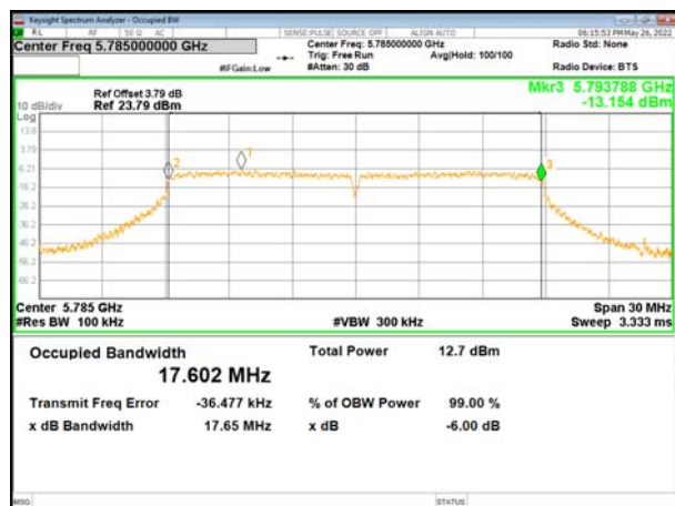
(802.11ac20) plot on channel 165
