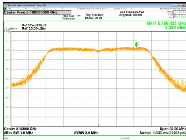
(802.11n20) PSD plot on channel 40
