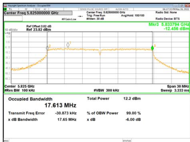
(802.11ac20) plot on channel 165
