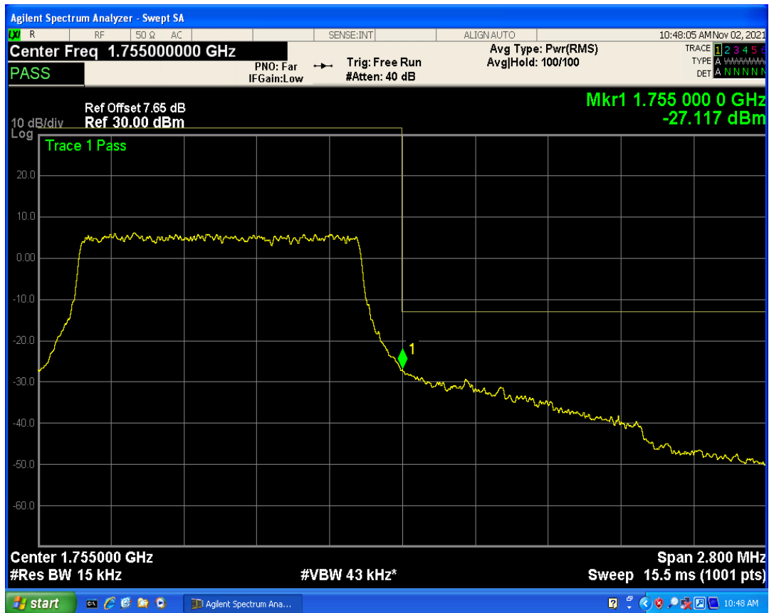
Band4 QPSK BW=1.4MHz Channel=20393 RB Size=1 Position=#Max
