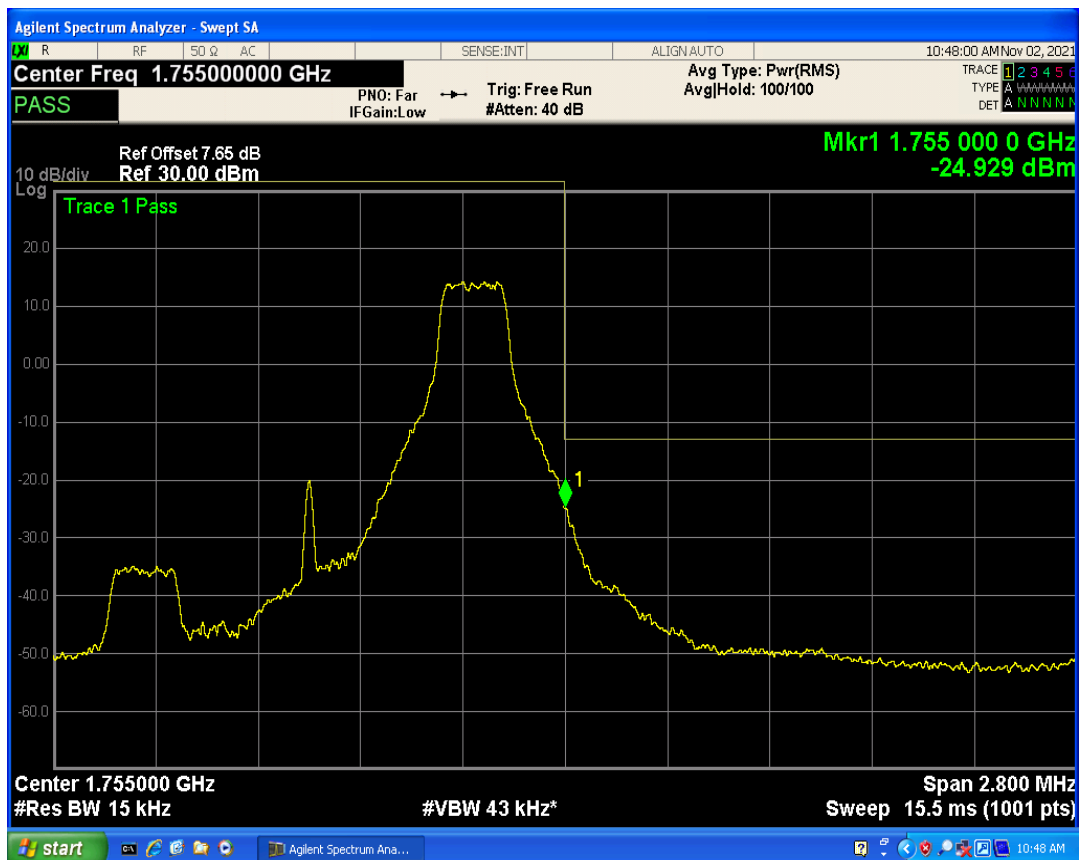
Band5 QAM16 BW=1.4MHz Channel=20407 RB Size=5 Position=#0
