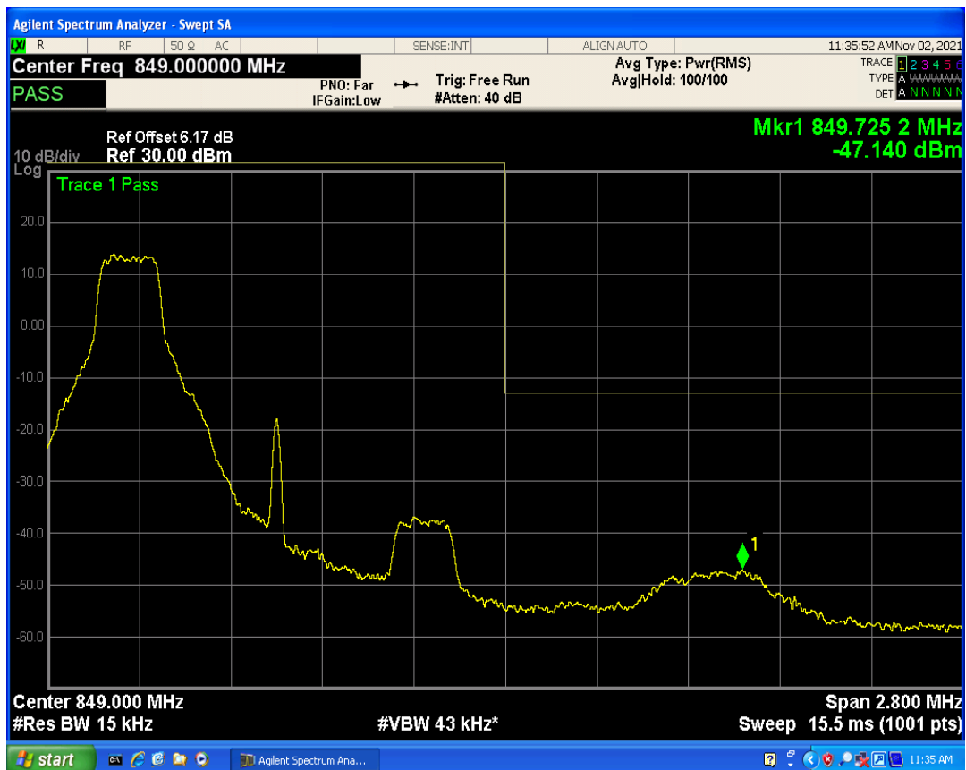
Band5 QPSK BW=1.4MHz Channel=20643 RB Size=1 Position=#Max
