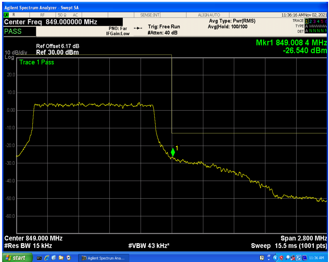
Band5 QAM16 BW=1.4MHz Channel=20643 RB Size=1 Position=#Max
