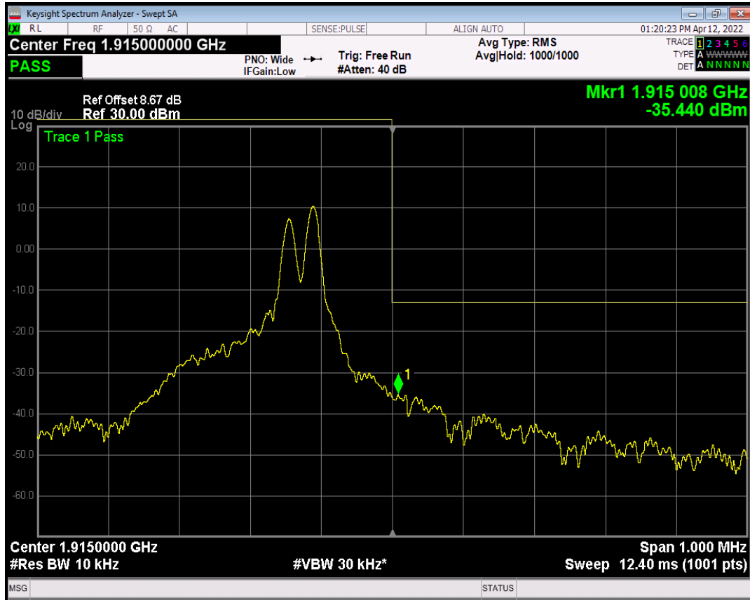
Band25 BPSK Channel=26688 nTones=1@11 Spacing=15kHz
