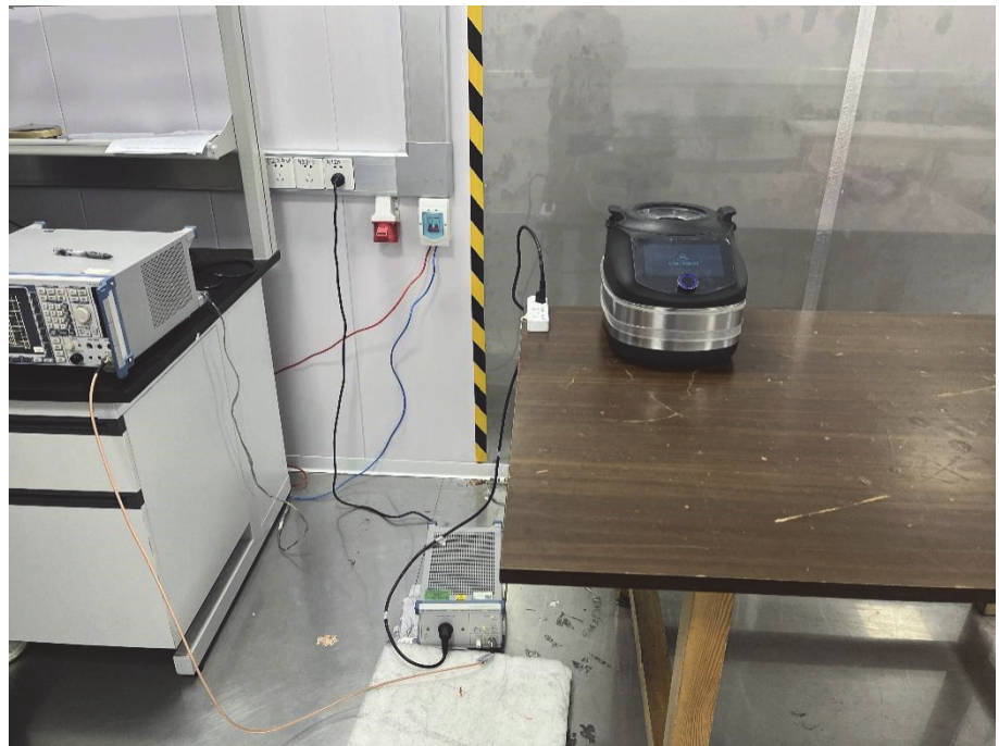
Conducted Emission Test Setup
