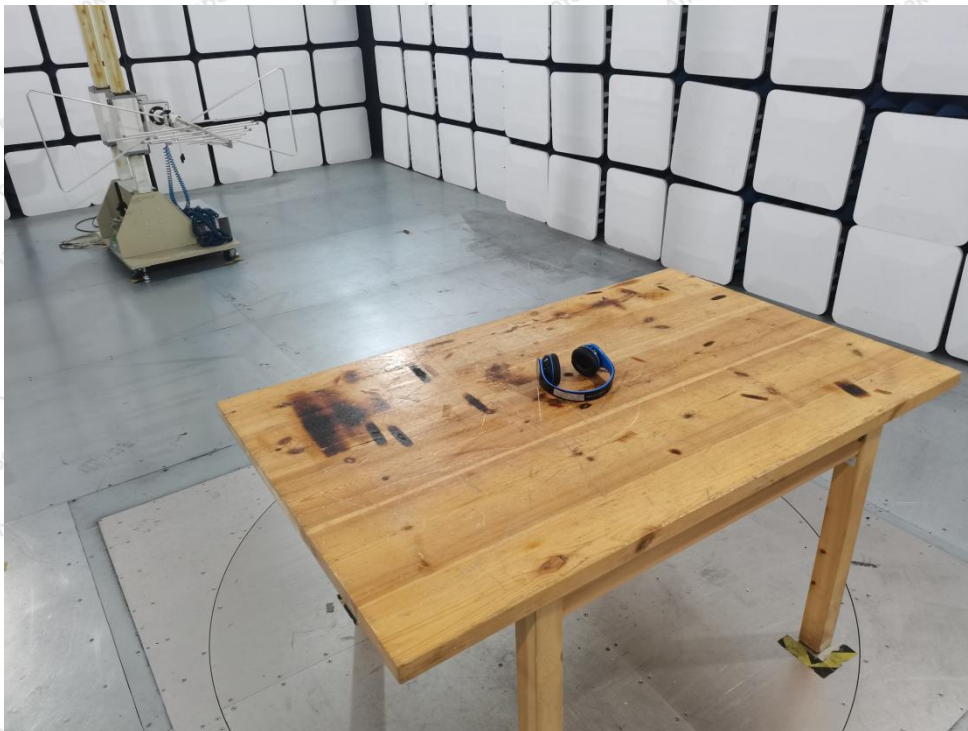
Photo of Radiation Emission Test
