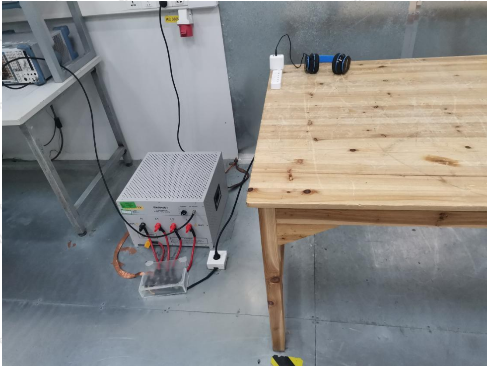
Photo of Conducted Emission Measurement
