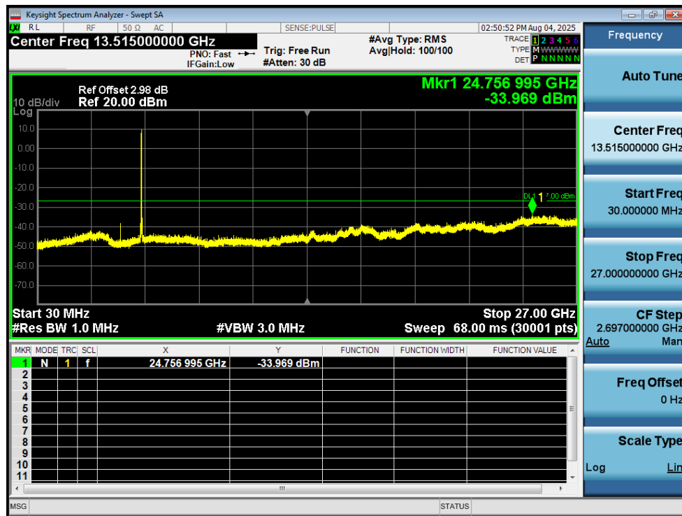
Tx. Spurious NVNT a 5240MHz Ant1 Emission
