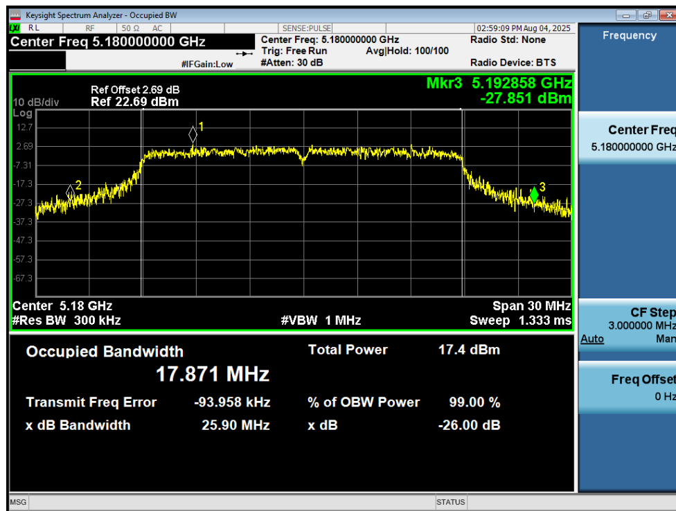
-26dB Bandwidth NVNT n20 5180MHz Ant1
