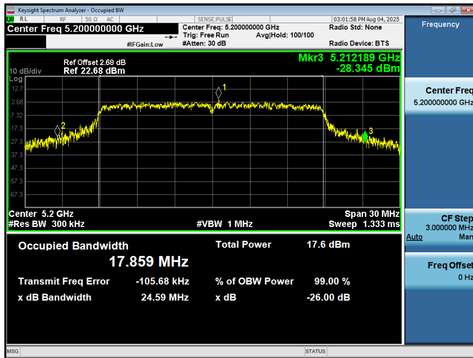
-26dB Bandwidth NVNT n20 5200MHz Ant1
