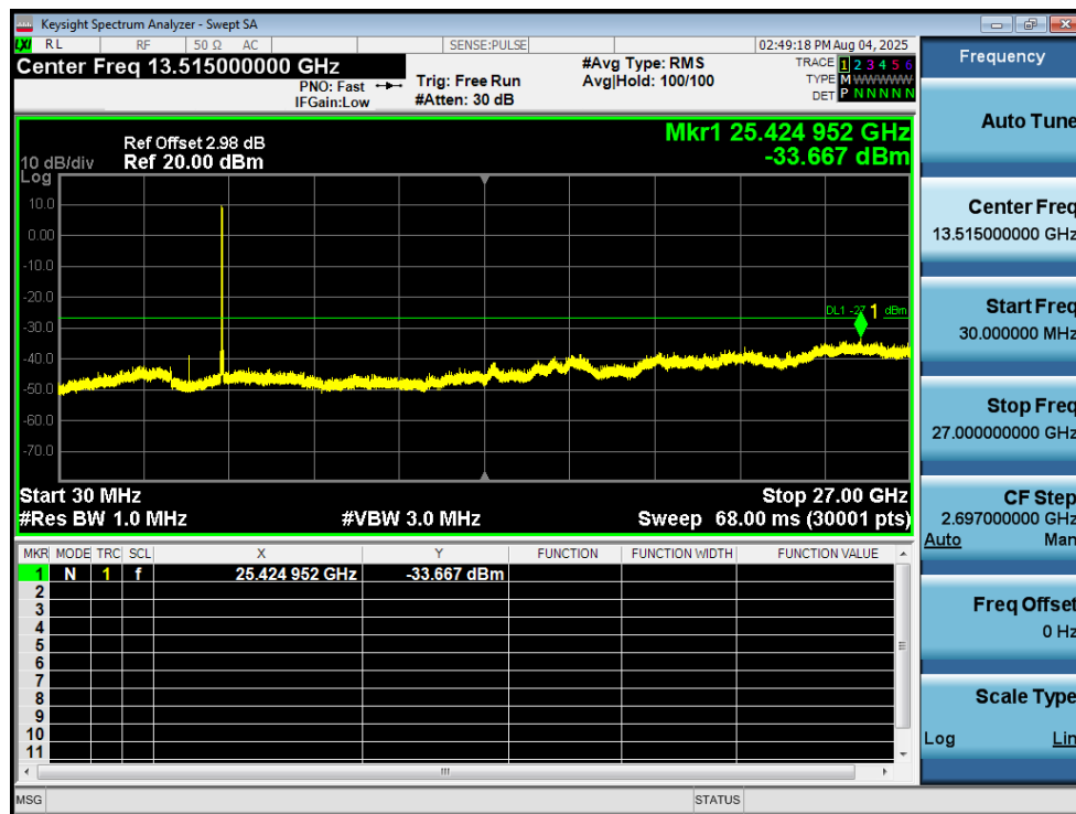
Tx. Spurious NVNT ac20 5200MHz Ant1 Emission
