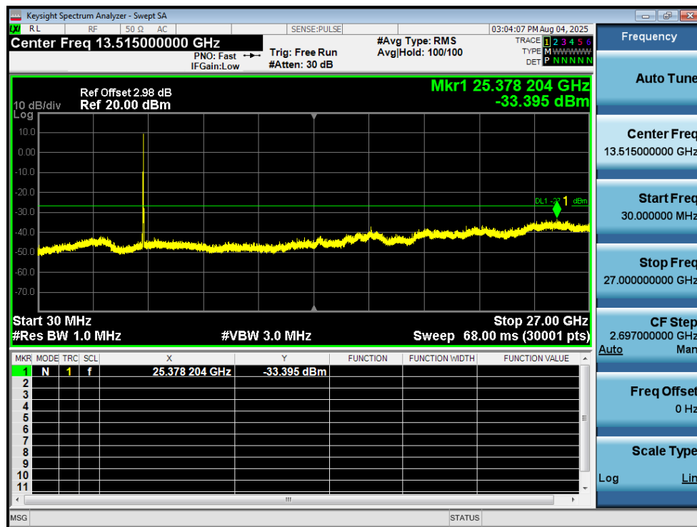
Tx. Spurious NVNT n20 5180MHz Ant1 Emission
