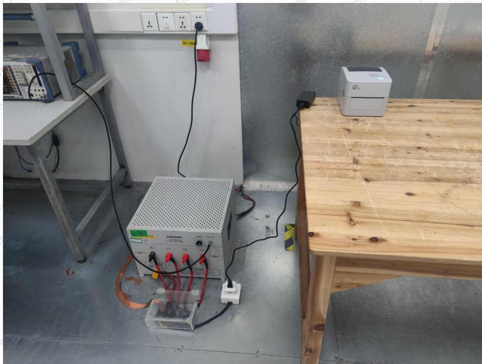
Photo of Conducted Emission Measurement
