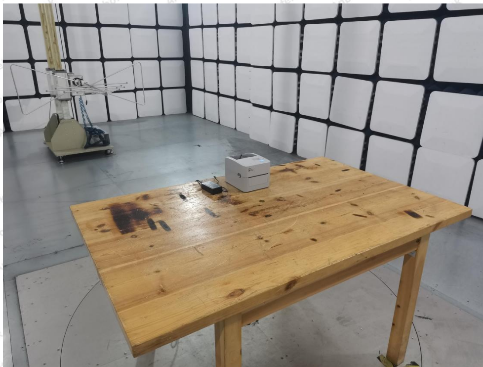
Photo of Radiation Emission Test
