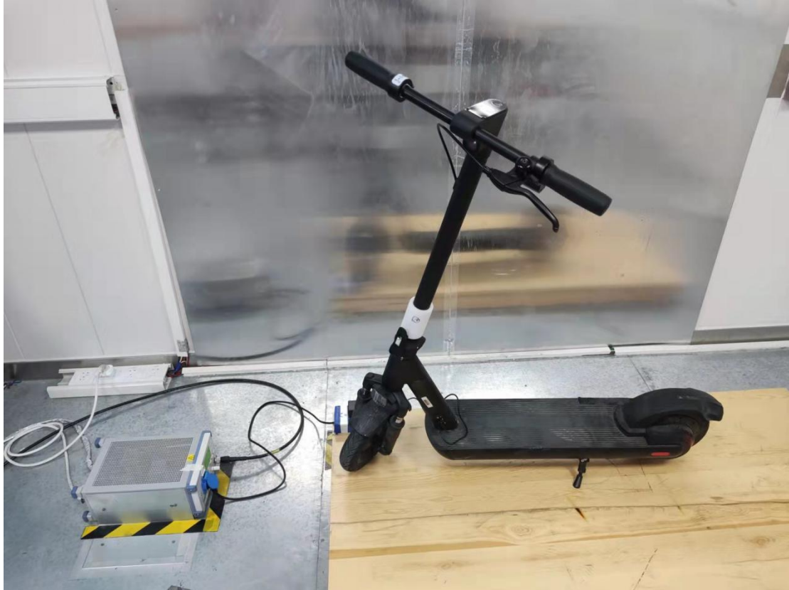
Conducted emission test setup
