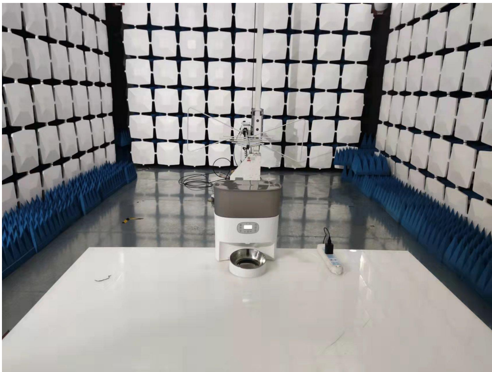
Below 1GHz for radiated emission test setup
