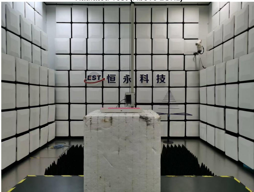
Radiated Test (Above 1GHz)
