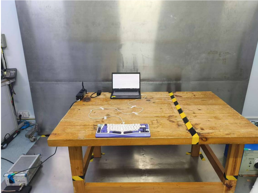
Conducted Emissions Side View
