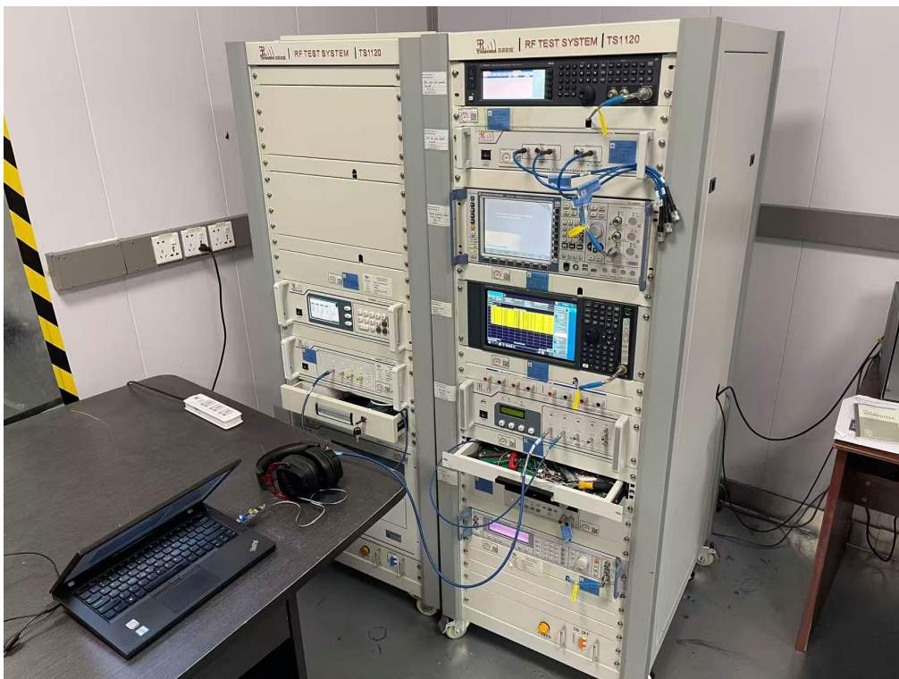
Connect EUT antenna terminal test
