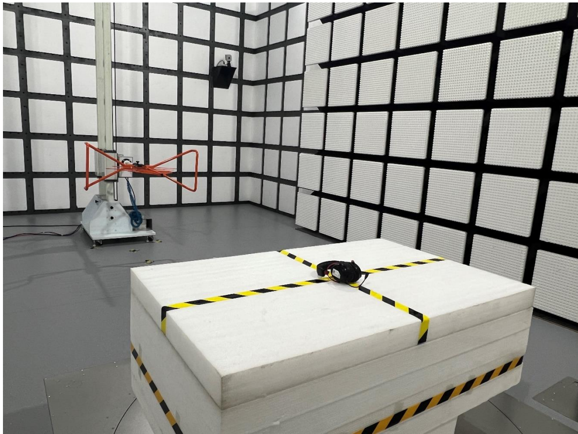
Radiated Emission 9 kHz-30 MHz Parallel View
