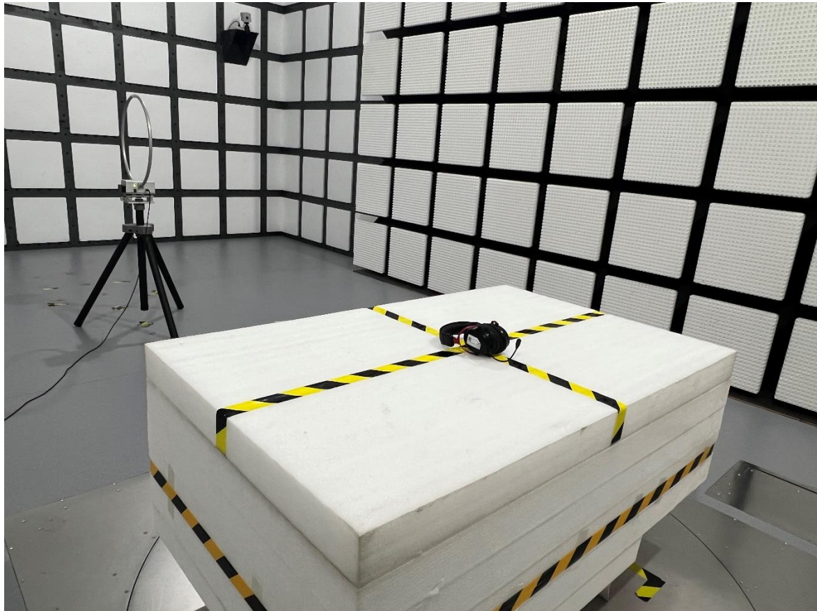
Radiated Emission 9 kHz-30 MHz Ground-parallel View
