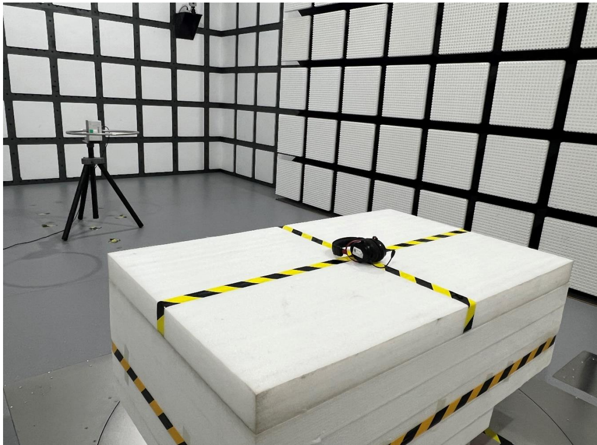
Radiated Emission 9 kHz-30 MHz Ground-parallel View
