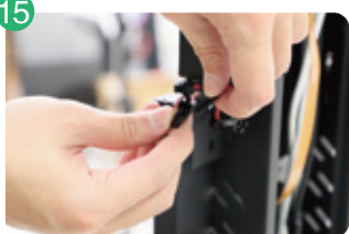
Step15: Connect wires between light bars
