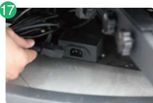
Step17: Connect power cable under the base
