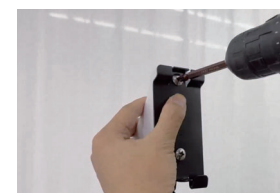
Step 8: Remove the back plate on Swivel Bracket and install it to Ring Light Bracket
