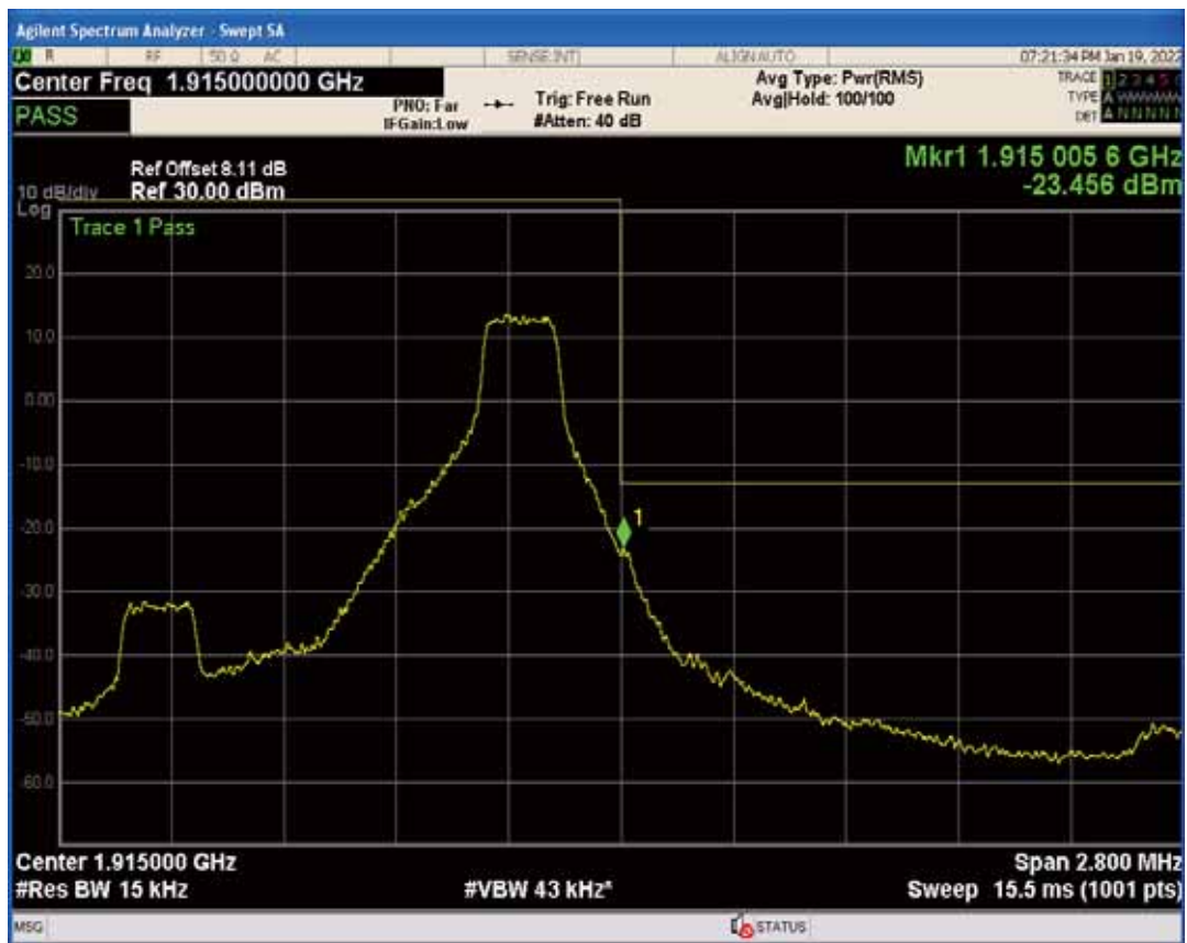
Band25 QPSK BW=10MHz Channel=26090 RB Size=1 Position=#Max
