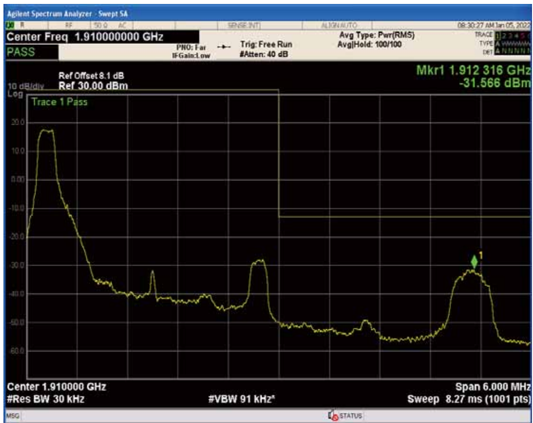
Band2 QPSK BW=3MHz Channel=19185 RB Size=1 Position=#Max
