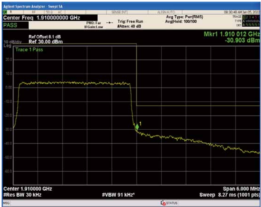
Band2 QPSK BW=5MHz Channel=18625 RB Size=1 Position=#0
