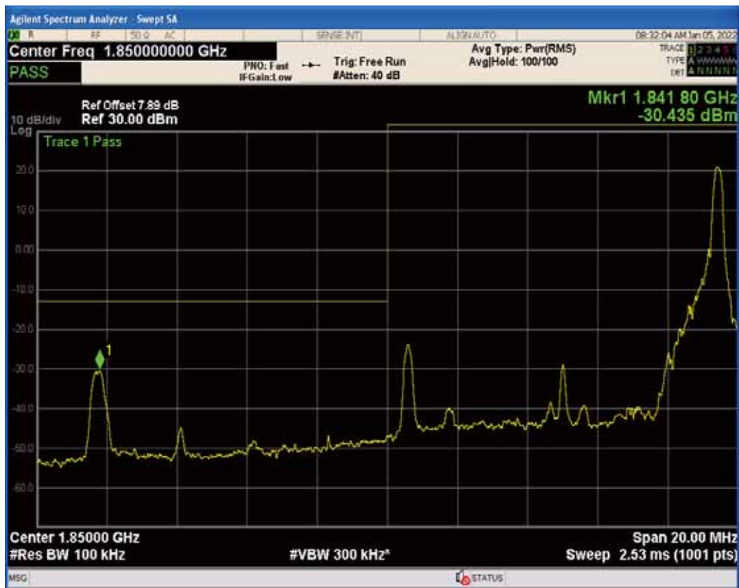
Band2 QPSK BW=10MHz Channel=19150 RB Size=1 Position=#0
