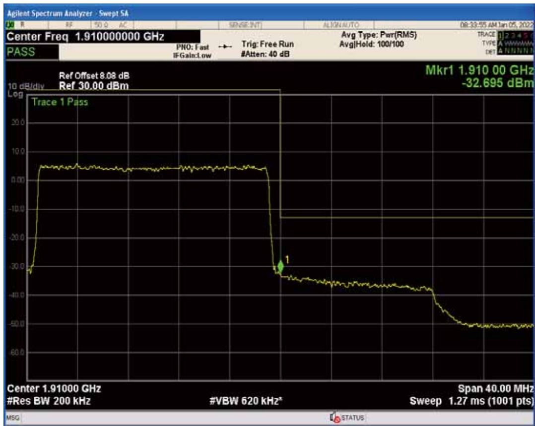
Band2 QAM16 BW=20MHz Channel=19100 RB Size=1 Position=#Max
