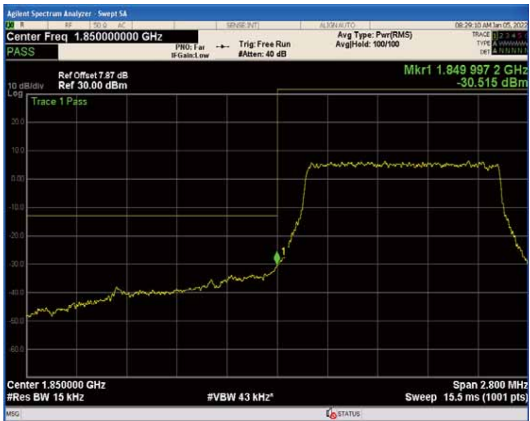
Band2 QAM16 BW=1.4MHz Channel=18607 RB Size=1 Position=#0
