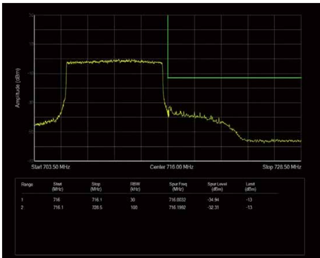
Band17 QAM16 BW=10MHz Channel=23800 RB Size=1 Position=#0
