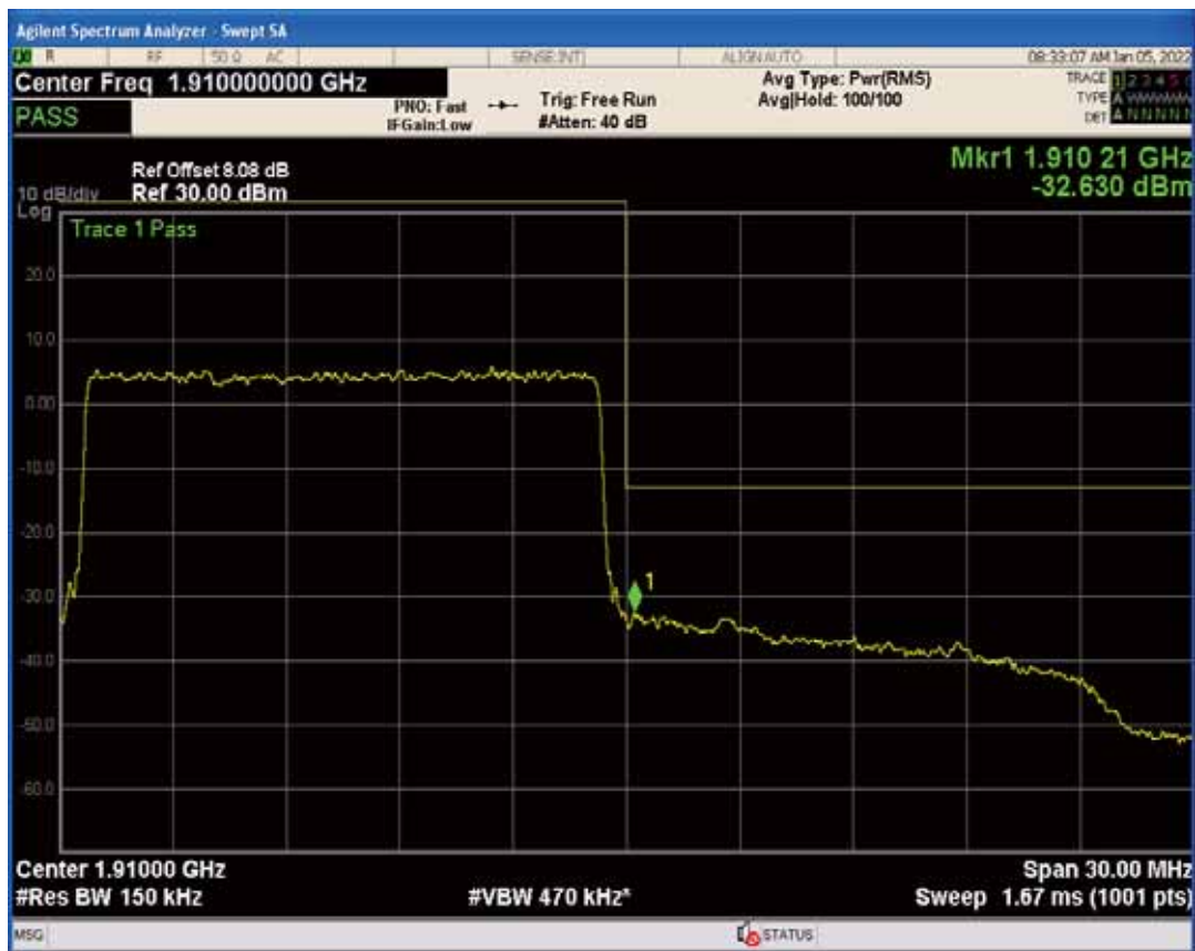
Band2 QAM16 BW=15MHz Channel=19125 RB Size=1 Position=#Max
