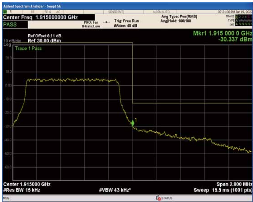
Band25 QPSK BW=1.4MHz Channel=26047 RB Size=1 Position=#0
