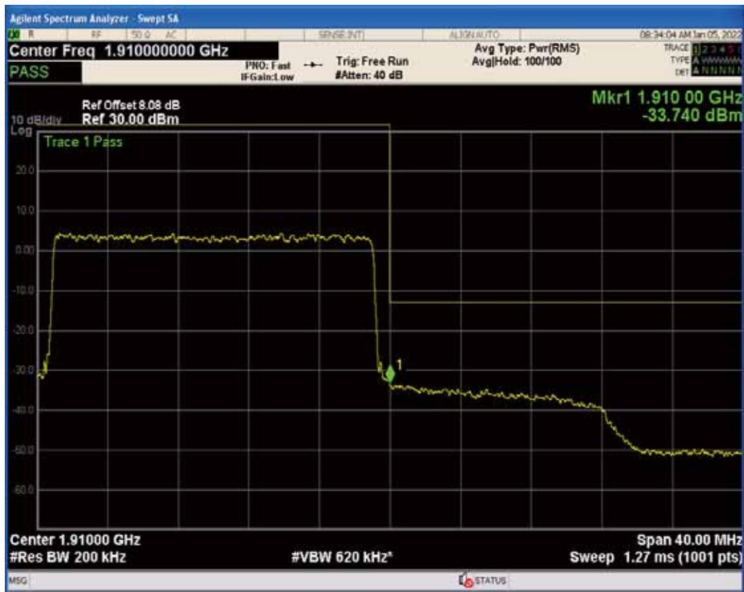
Band25 QAM16 BW=10MHz Channel=26090 RB Size=50 Position=#0
