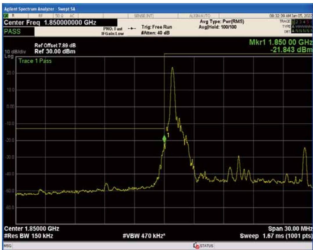
Band2 QAM16 BW=10MHz Channel=19150 RB Size=50 Position=#0
