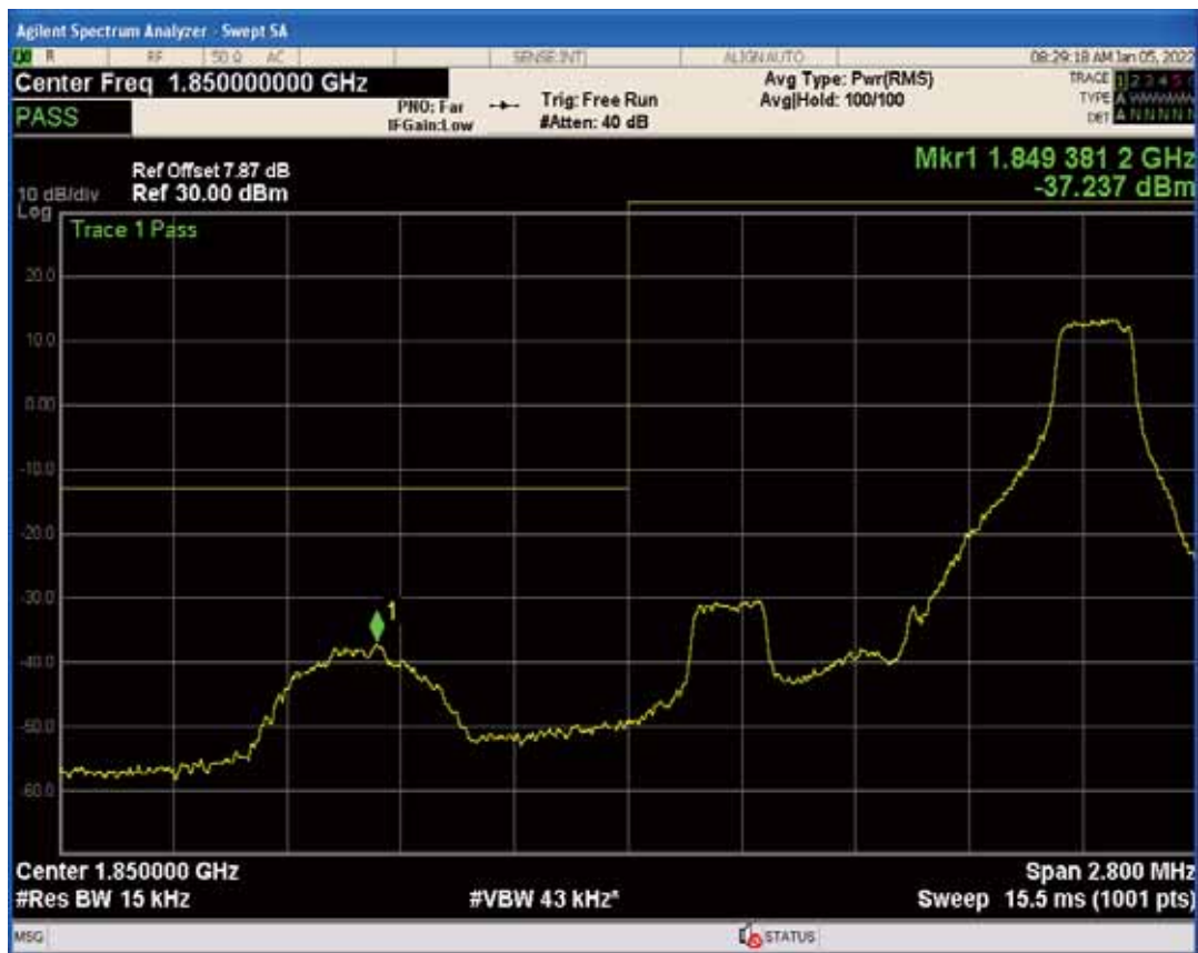
Band2 QPSK BW=1.4MHz Channel=19193 RB Size=1 Position=#0
