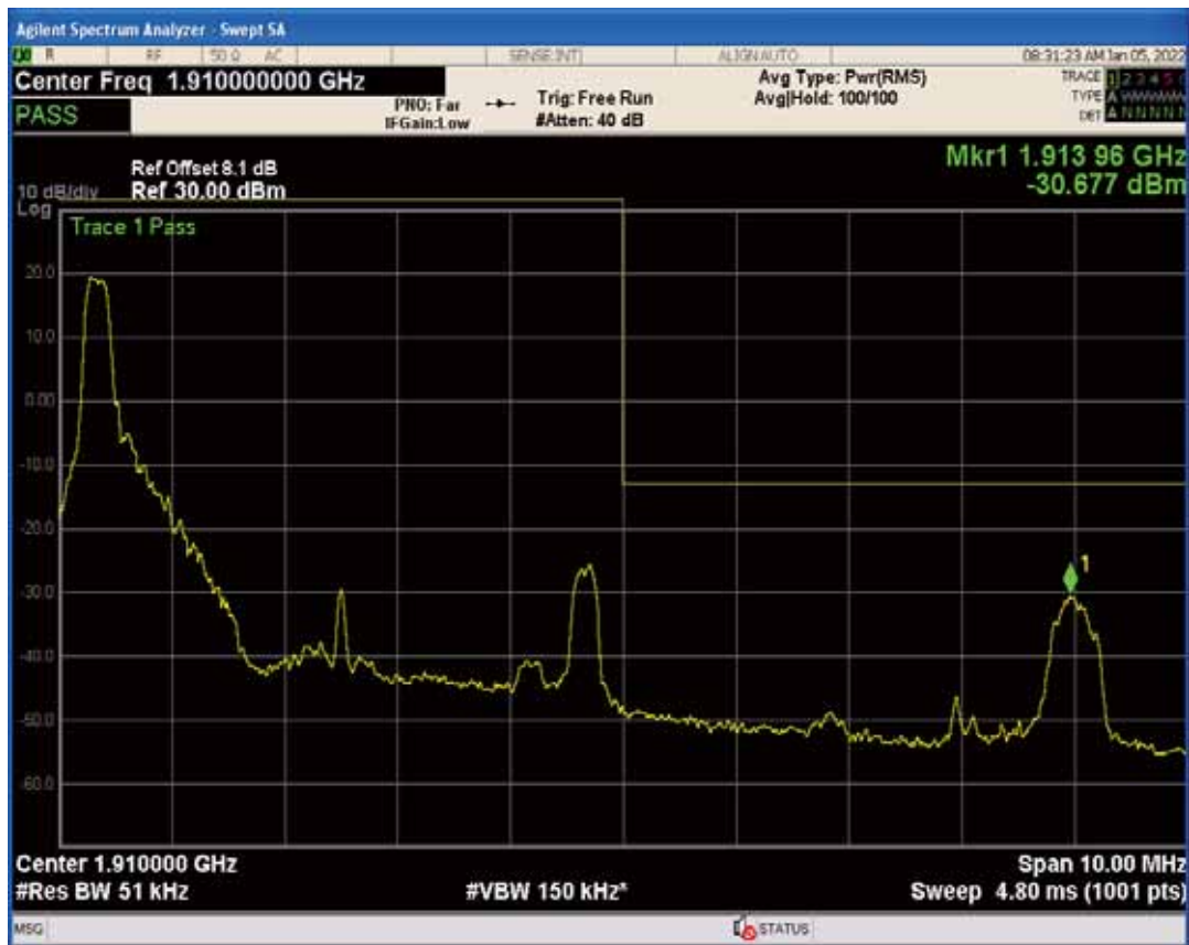
Band2 QPSK BW=5MHz Channel=19175 RB Size=25 Position=#0
