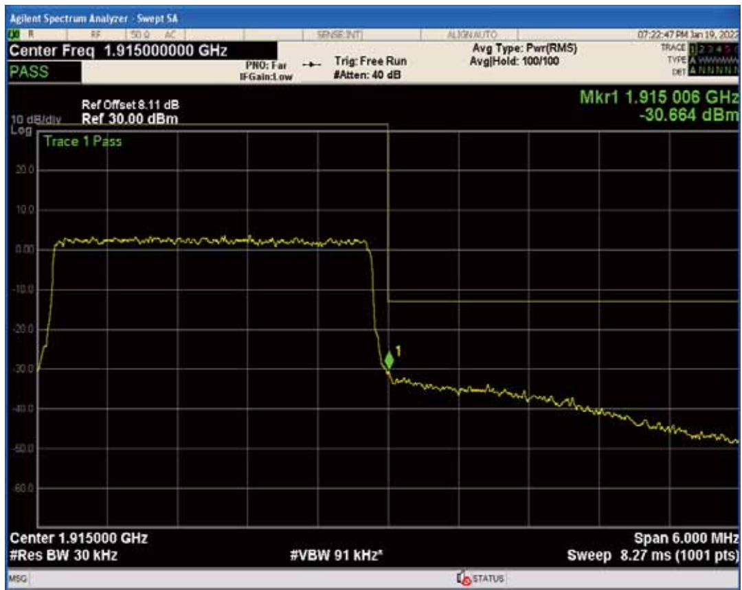
Band25 QAM16 BW=5MHz Channel=26065 RB Size=25 Position=#0
