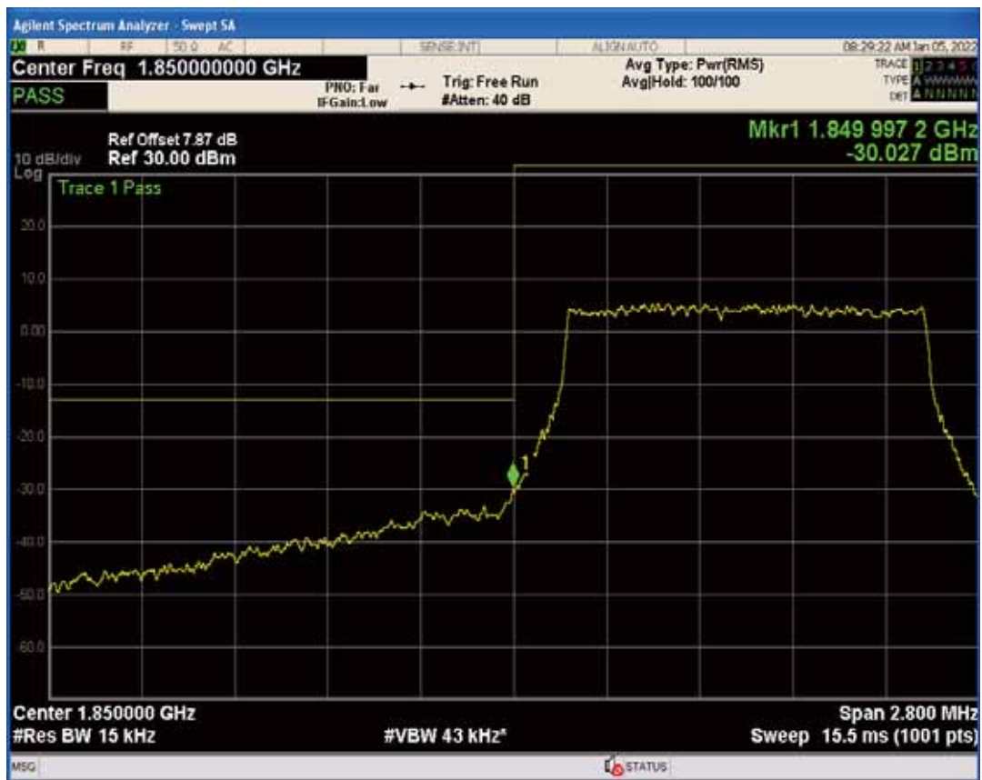
Band2 QPSK BW=1.4MHz Channel=19193 RB Size=1 Position=#Max
