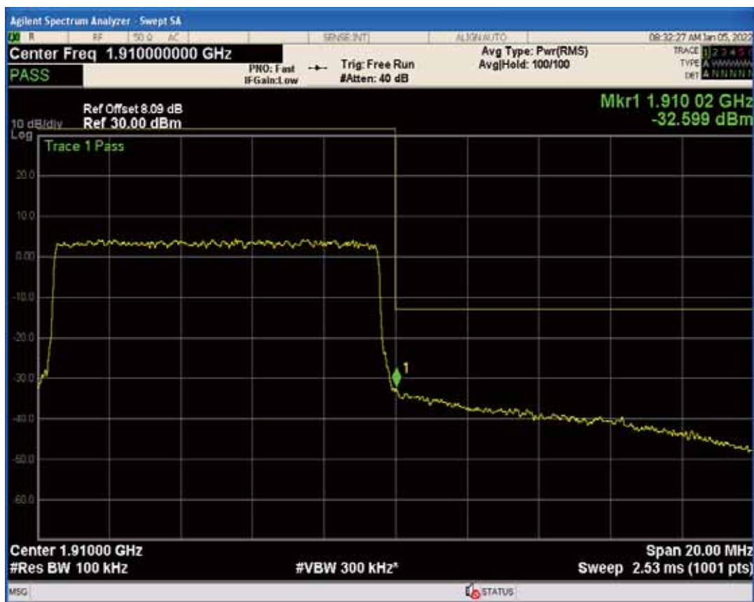
Band2 QPSK BW=15MHz Channel=18675 RB Size=75 Position=#0
