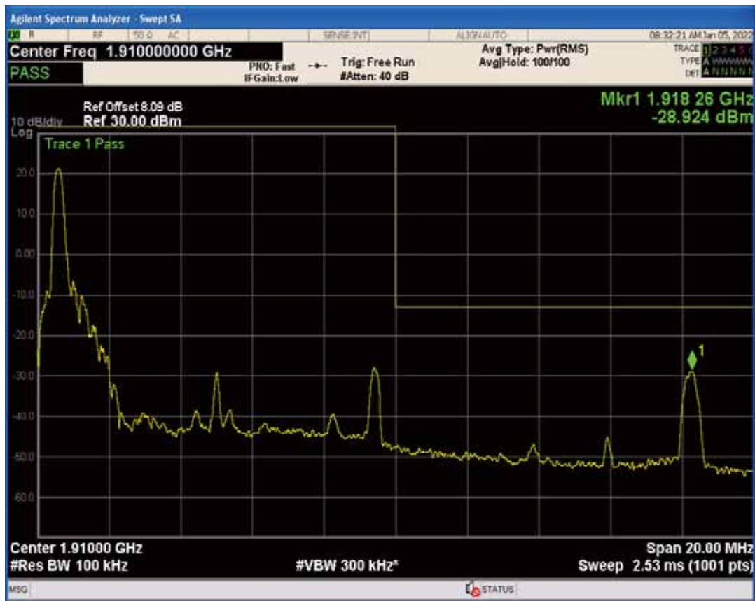
Band2 QAM16 BW=10MHz Channel=19150 RB Size=1 Position=#Max
