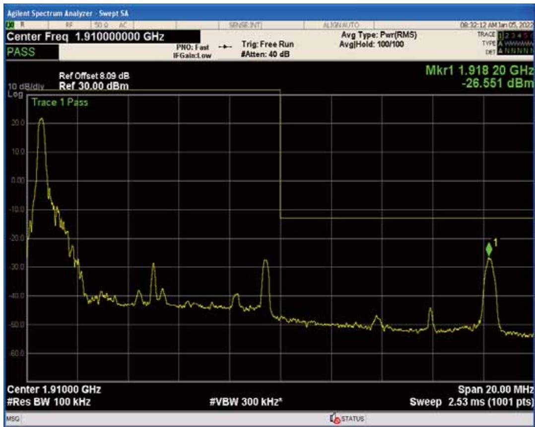
Band2 QAM16 BW=10MHz Channel=18650 RB Size=50 Position=#0
