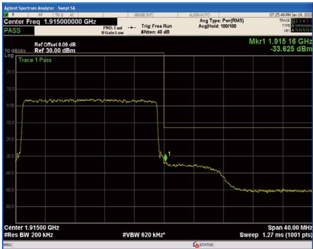
Band25 QPSK BW=3MHz Channel=26055 RB Size=1 Position=#0
