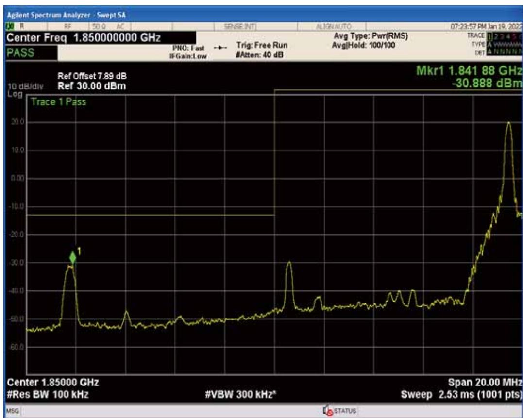
Band25 QAM16 BW=10MHz Channel=26090 RB Size=1 Position=#0
