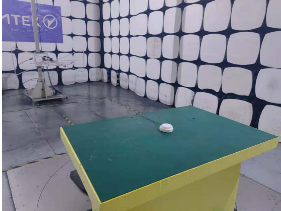
Spurious Emission Test Setup (Above 1GHz)
