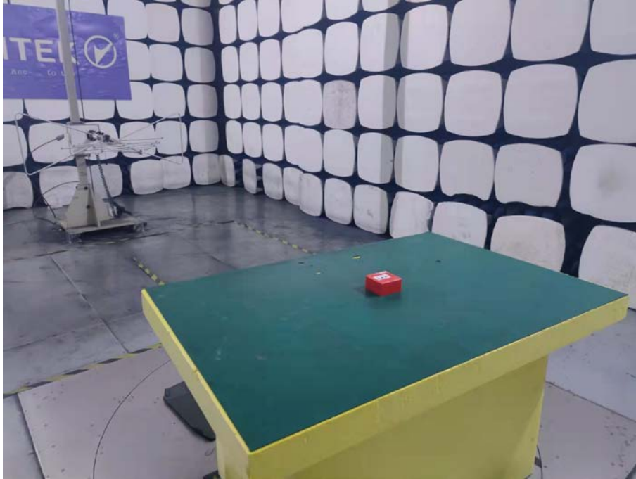
Spurious Emission Test Setup (Above 1GHz)
