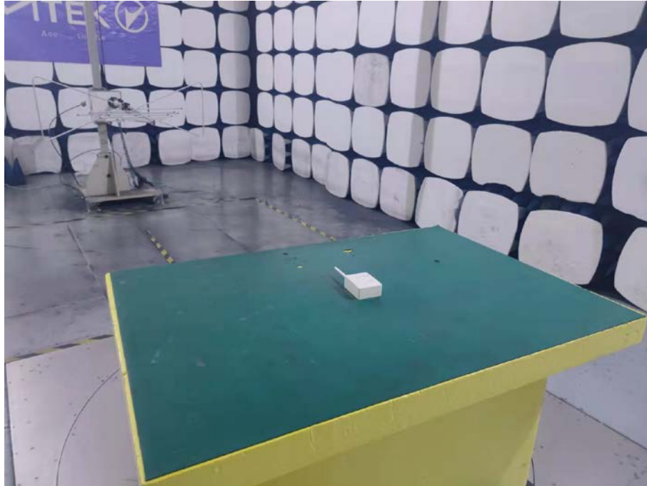
Spurious Emission Test Setup (Above 1GHz)
