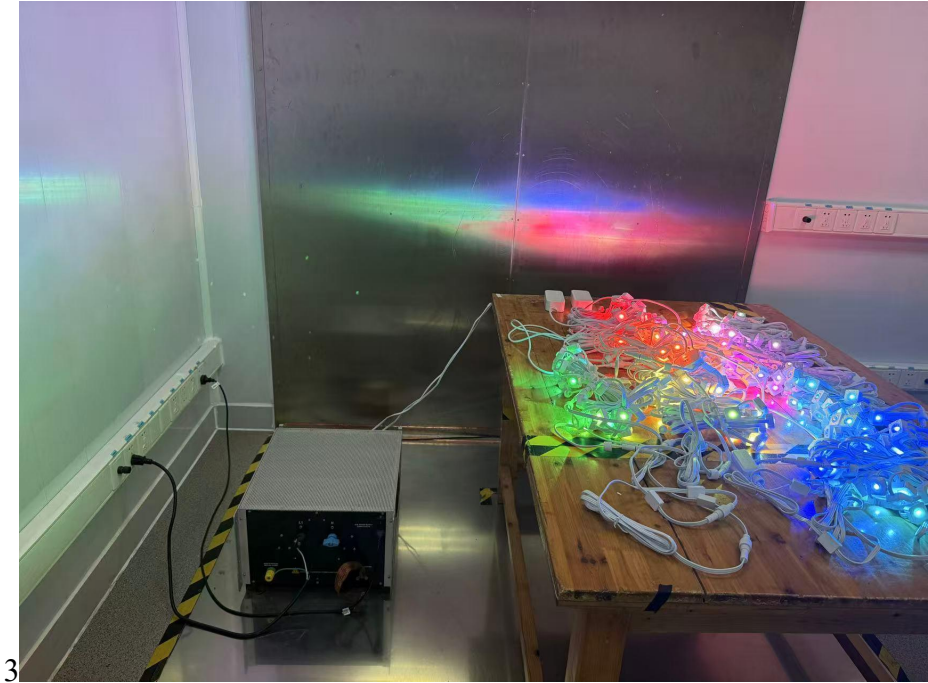
Photos of Conducted Emission Test
