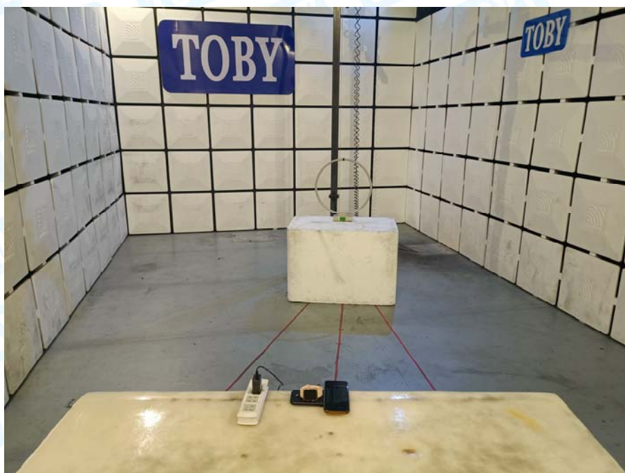
Photo of Setup for Radiated Emission (9KHz-30MHz)
