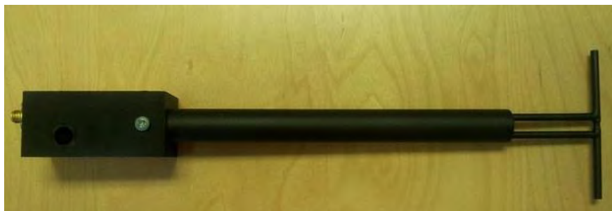
Figure 1 – MVG COMOSAR Validation Dipole
