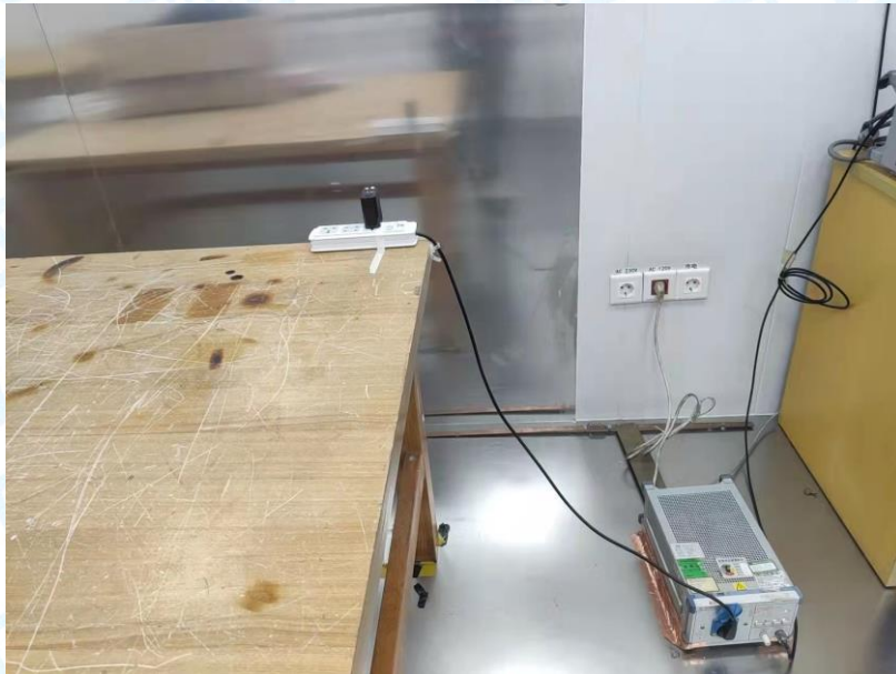
Photo of Setup for Conducted Emission
