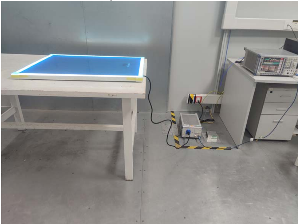
Photos of radiated emission test 30MHz – 1GHz
