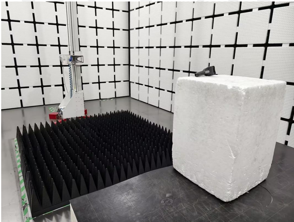
Spurious Radiation Emissions Test (>1G)
