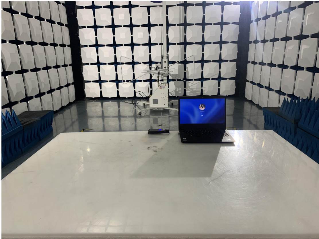
Above 1GHz for radiated emission test setup
