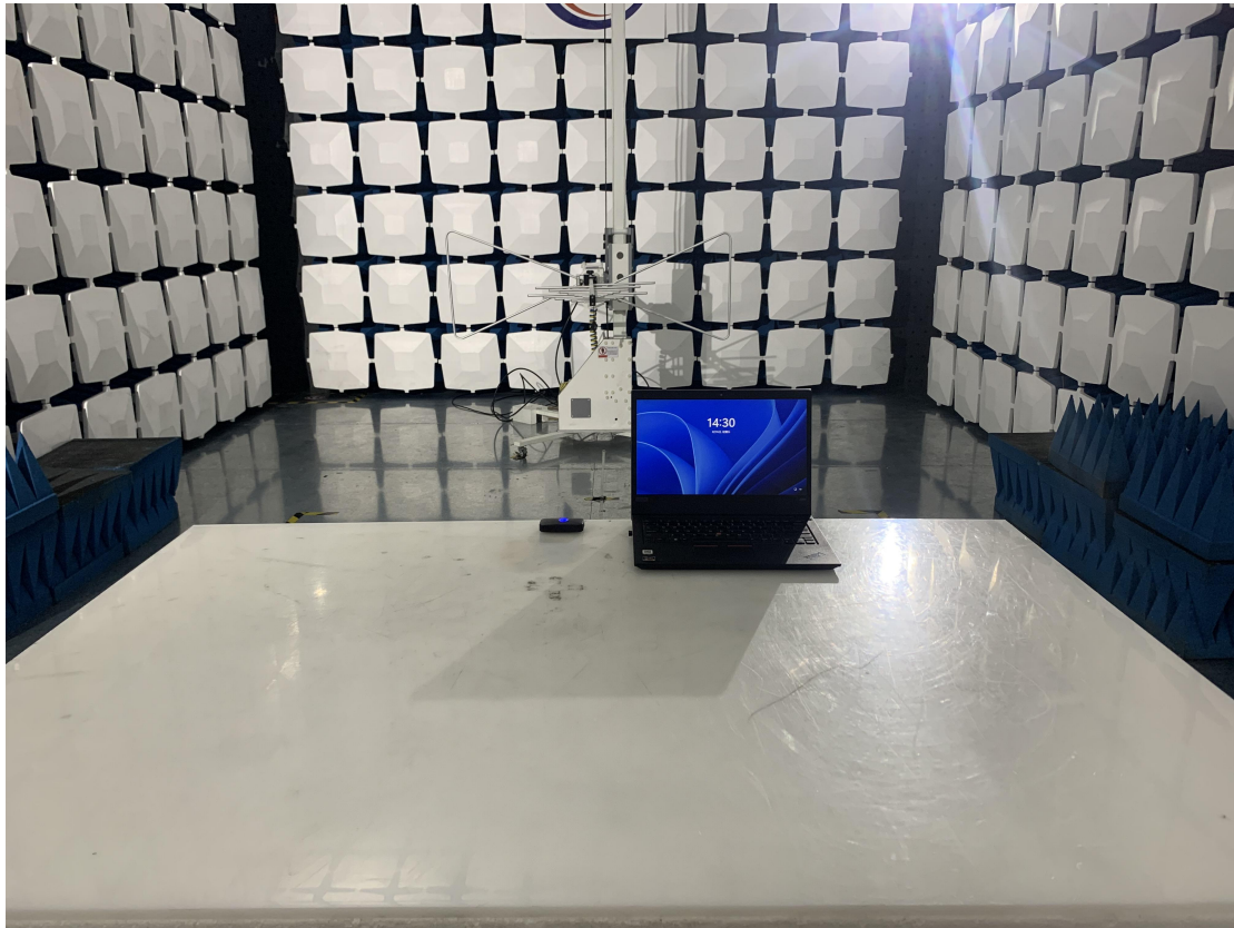
Above 1GHz for radiated emission test setup
