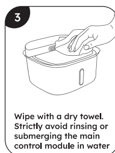
Maintenance of the main control module
