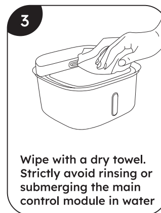
Maintenance of the main control module
