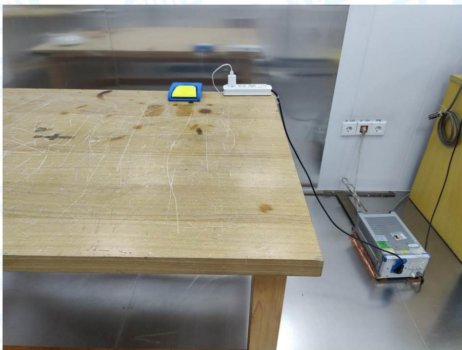
Photo of Setup for Conducted Emission
