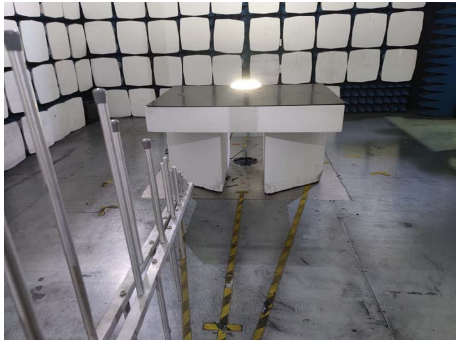
Radiation Emission Test Setup (30MHz to 1GHz)
