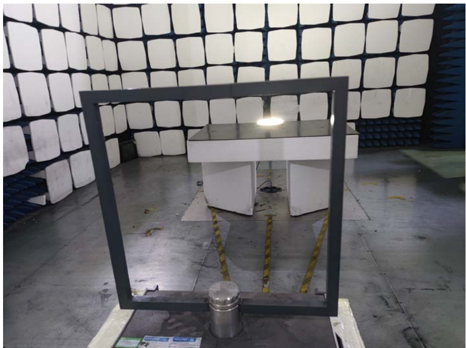
Radiation Emission Test Setup (Below 30MHz)
