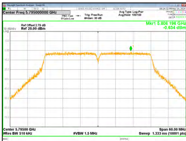
(802.11ac40) PSD plot on channel 159
