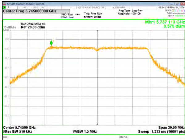
(802.11ac20) PSD plot on channel 149
