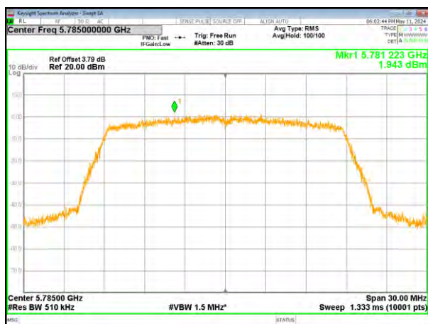
(802.11ac20) PSD plot on channel 157
