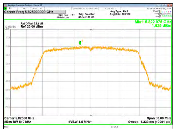
(802.11n20) PSD plot on channel 165
