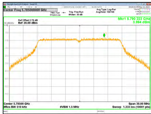
(802.11n20) PSD plot on channel 165
