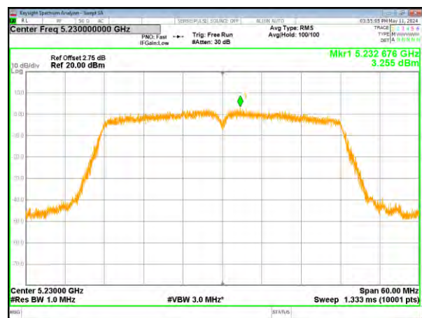
(802.11n40) PSD plot on channel 46
