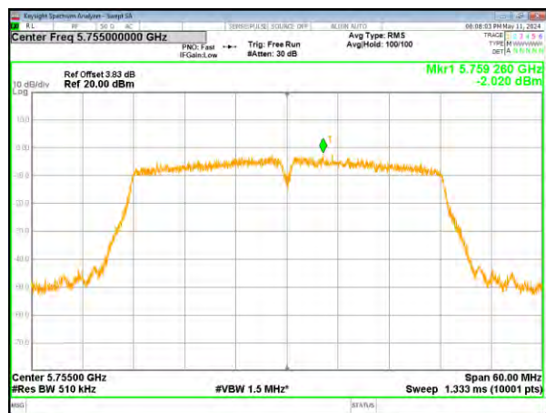
(802.11n40) PSD plot on channel 159
