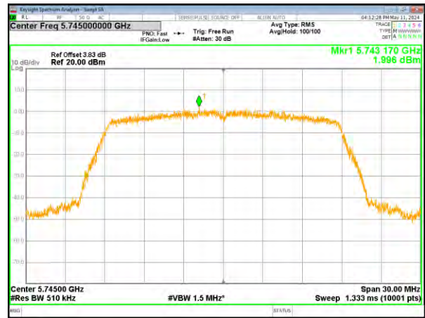
(802.11n20) PSD plot on channel 157
