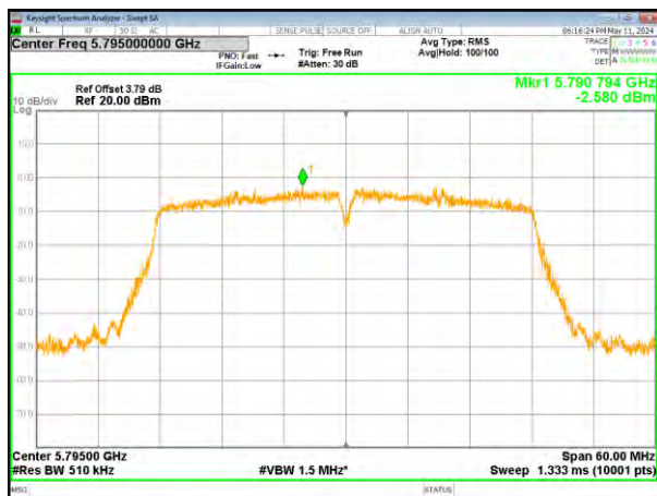
(802.11ac40) PSD plot on channel 159
