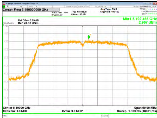
(802.11ac40) PSD plot on channel 46
