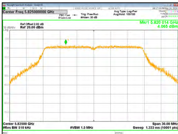
(802.11ac20) PSD plot on channel 165
