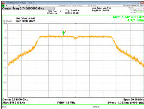
(802.11a) PSD plot on channel 157
