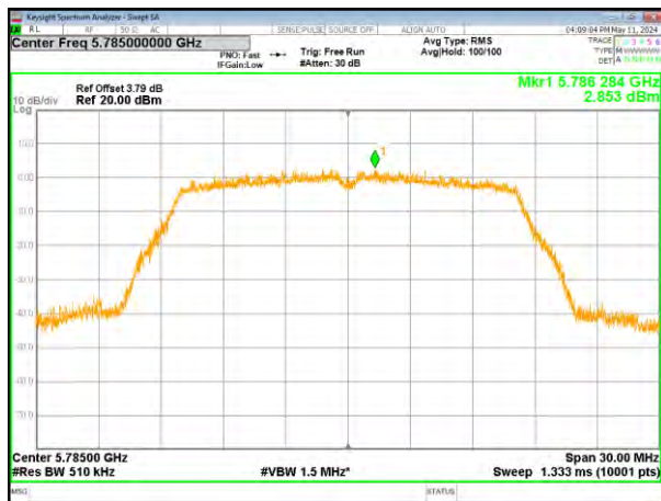
(802.11a) PSD plot on channel 157
