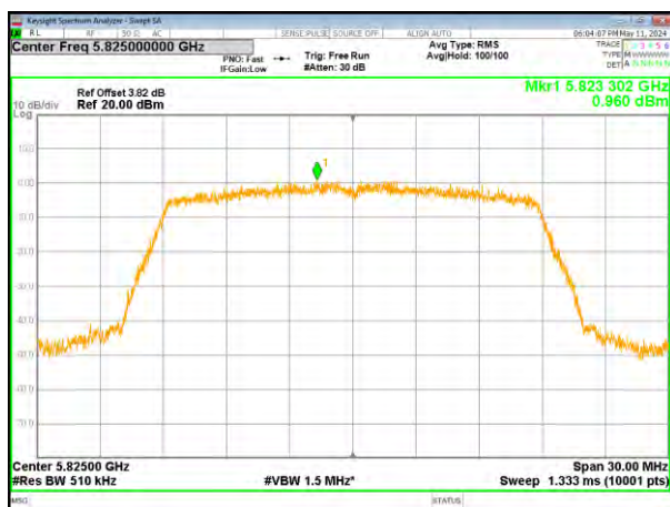
(802.11ac20) PSD plot on channel 165
