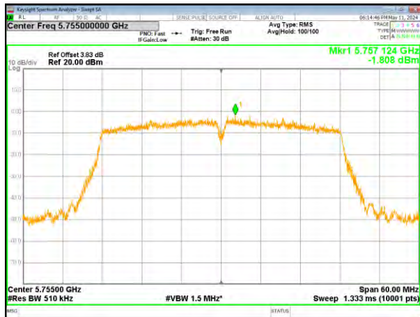
(802.11ac40) PSD plot on channel 151
