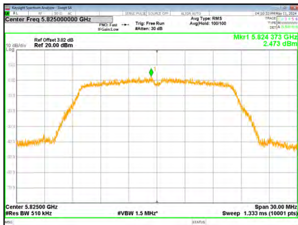
(802.11a) PSD plot on channel 165
