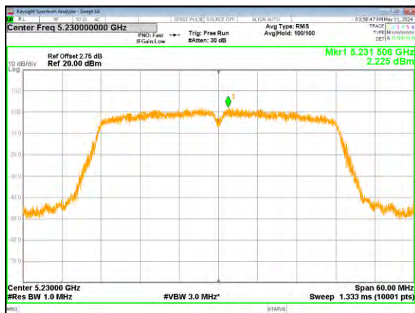
(802.11ac40) PSD plot on channel 46
