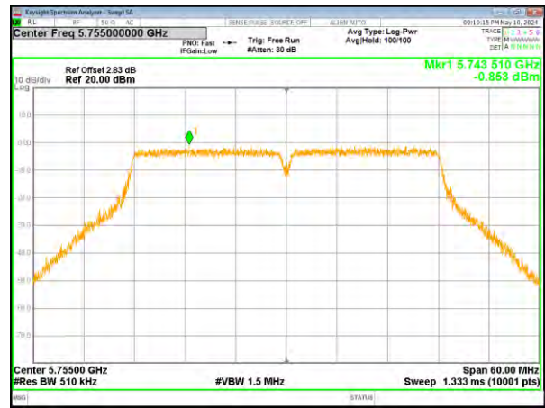
(802.11n40) PSD plot on channel 151
