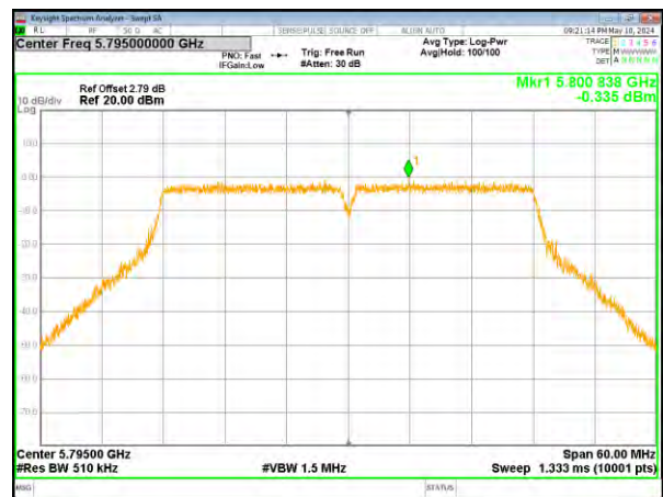
(802.11n40) PSD plot on channel 159
