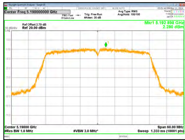
(802.11n40) PSD plot on channel 46
