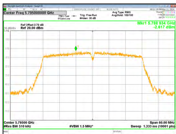
(802.11n40) PSD plot on channel 159
