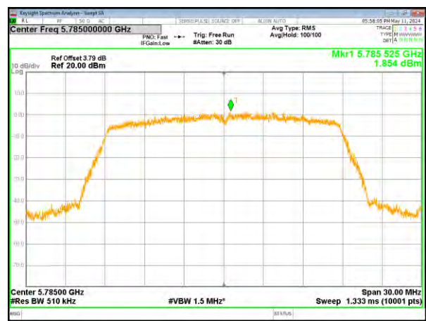
(802.11n20) PSD plot on channel 157
