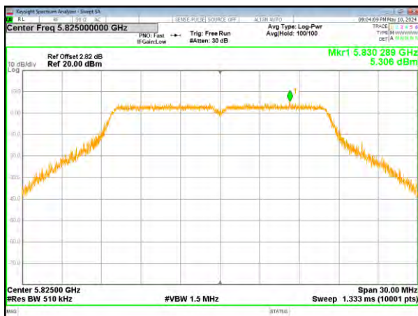
(802.11a) PSD plot on channel 165
