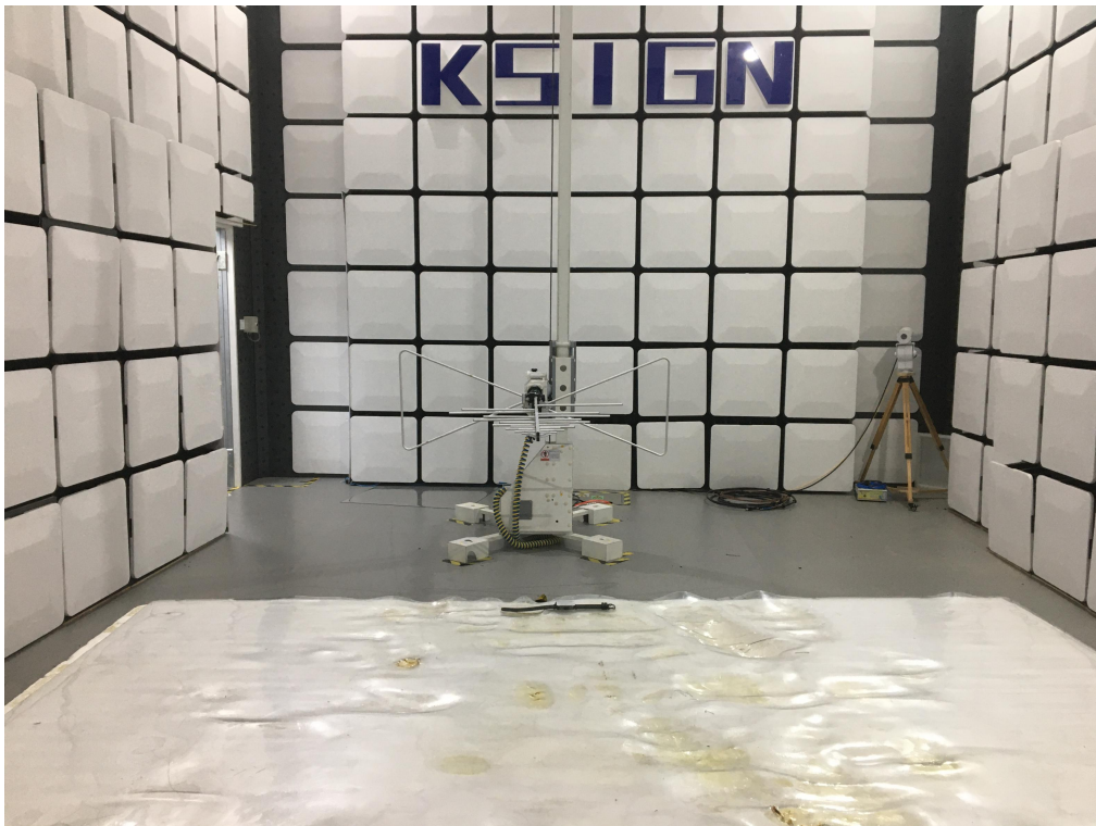
Radiated Measurement (Above 1GHz)
