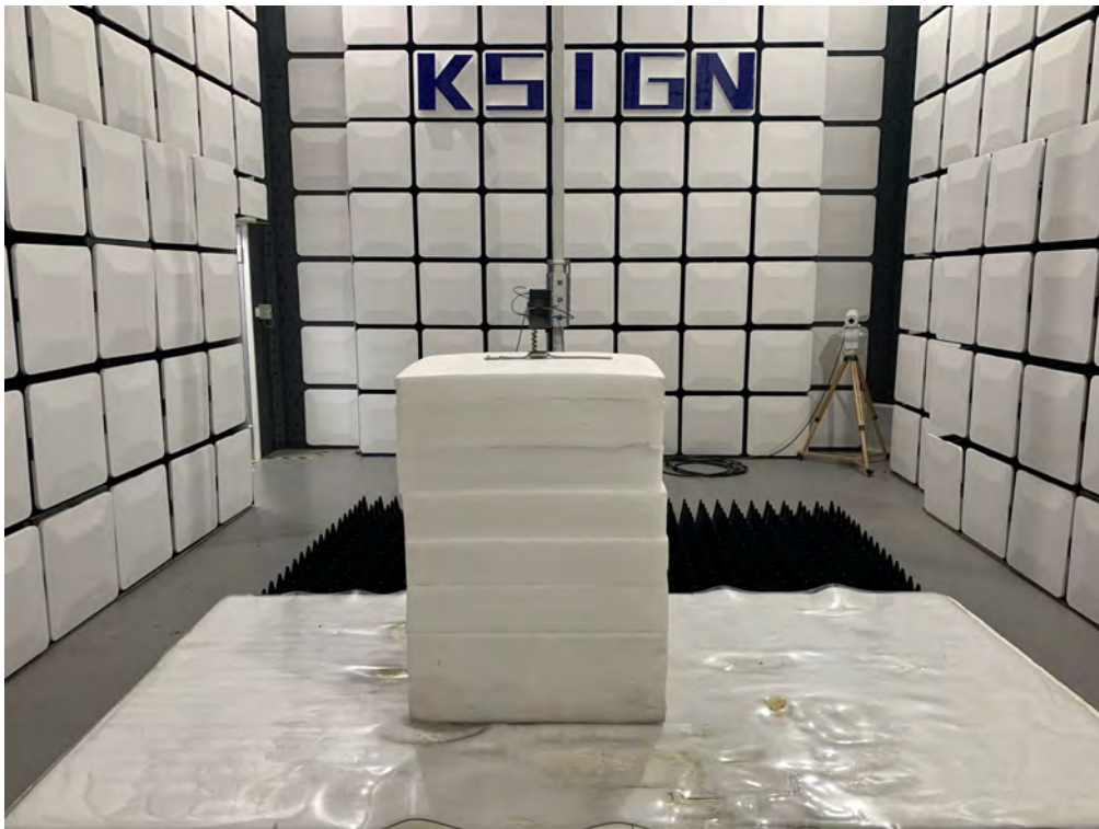
Radiated Measurement (Above 1GHz)
