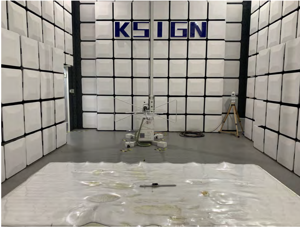
Radiated Measurement (Above 1GHz)
