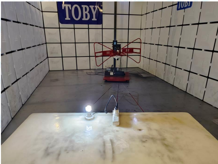
Photo of Setup for Conducted Emission
