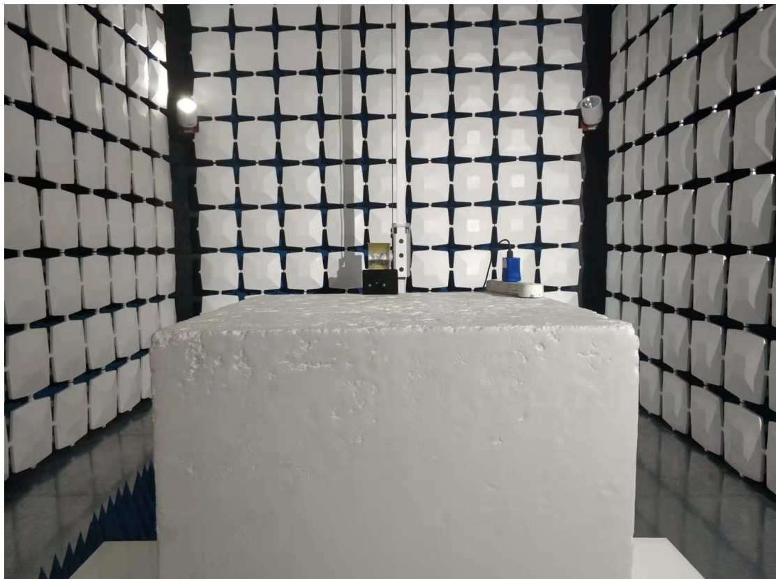
Above 1GHz for radiated emission test setup
