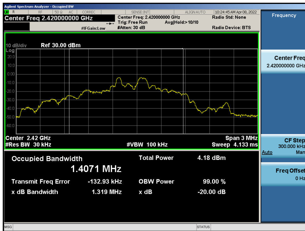
TEST PLOT OF BANDWIDTH FOR LOW CHANNEL
