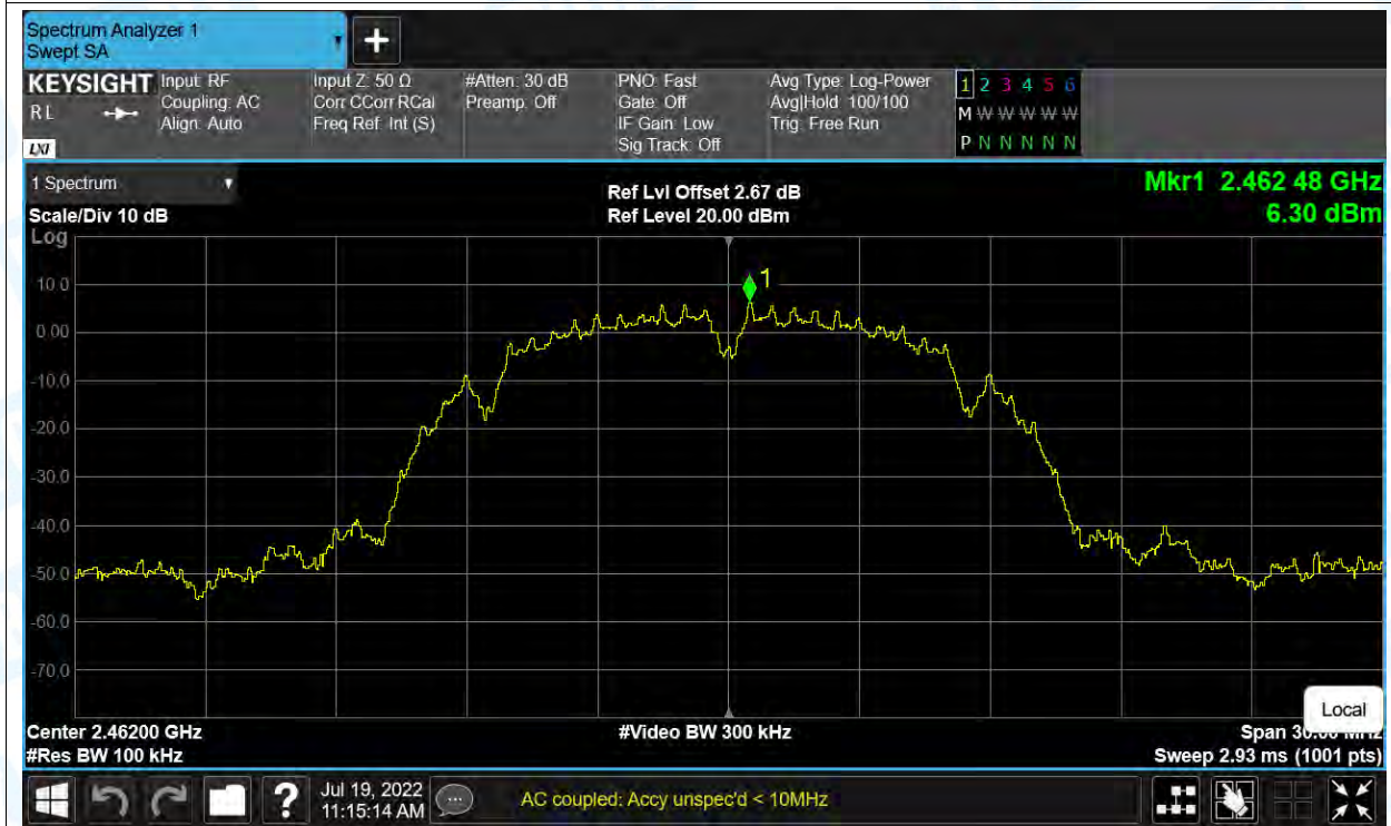
Tx. Spurious NVNT b 2462MHz Ant1 Emission
