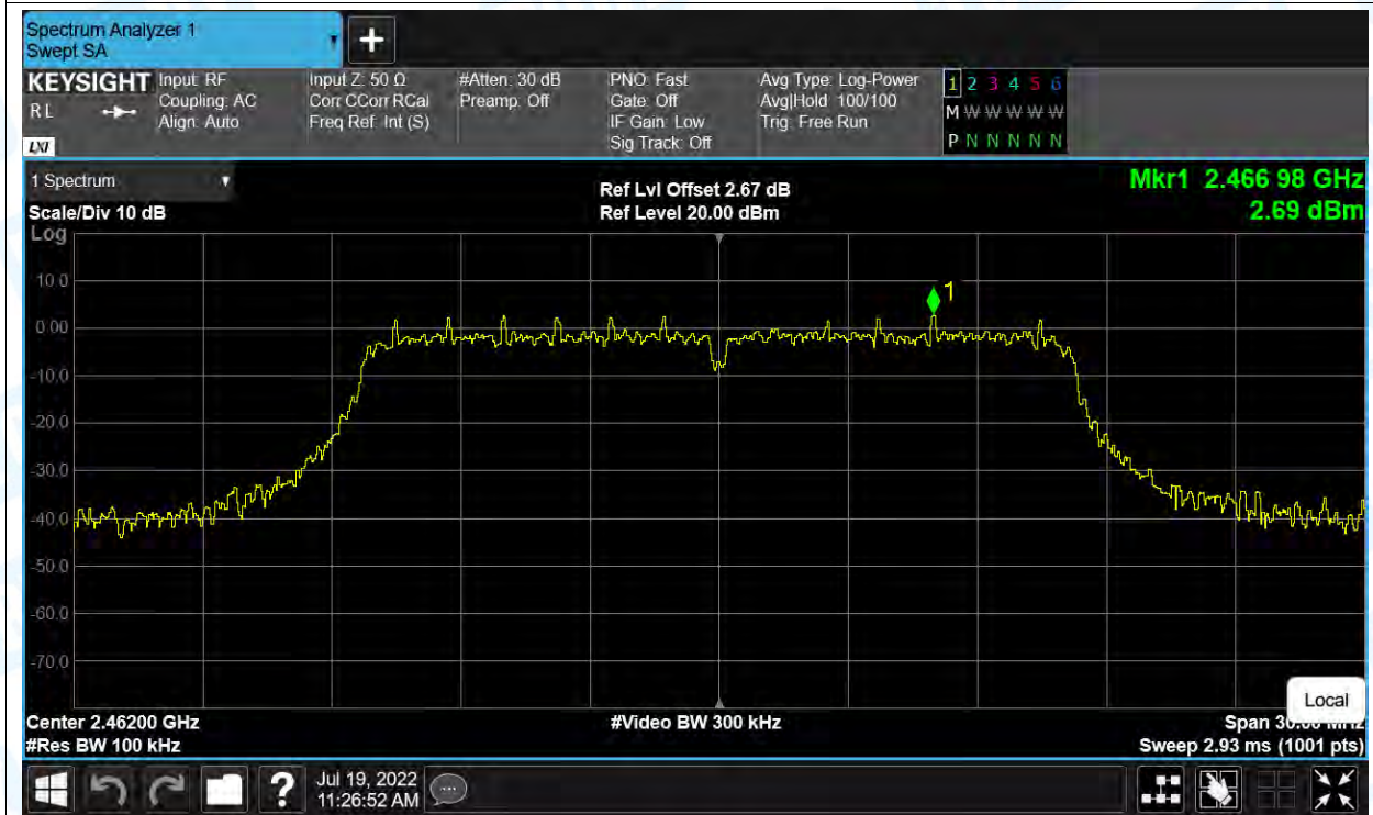
Tx. Spurious NVNT g 2462MHz Ant1 Emission
