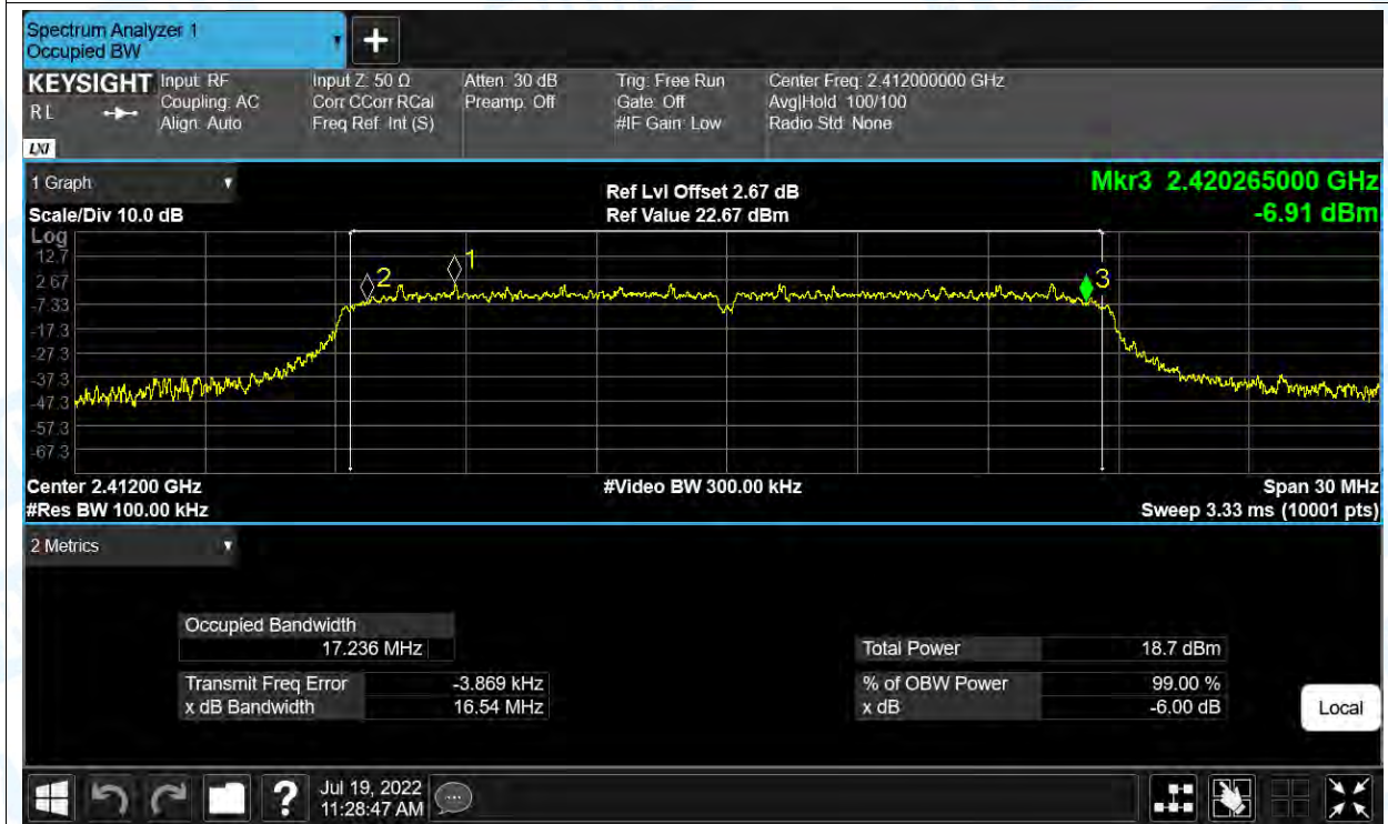
-6dB Bandwidth NVNT n(HT20) 2437MHz Ant1
