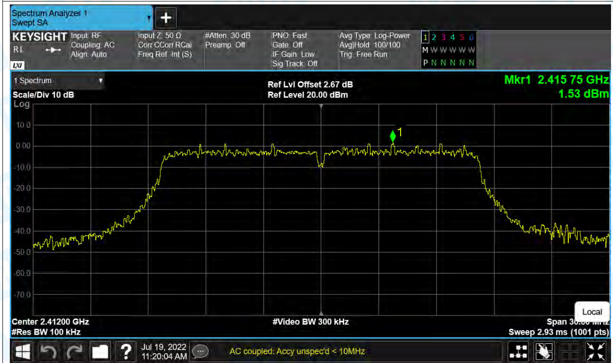
Tx. Spurious NVNT g 2412MHz Ant1 Emission
