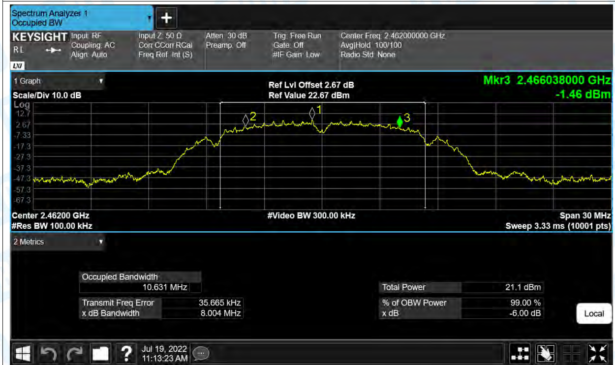
-6dB Bandwidth NVNT g 2412MHz Ant1
