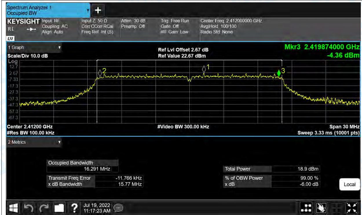
-6dB Bandwidth NVNT g 2412MHz Ant1
