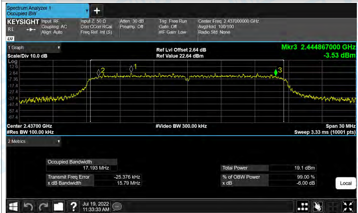
-6dB Bandwidth NVNT n(HT20) 2437MHz Ant1
