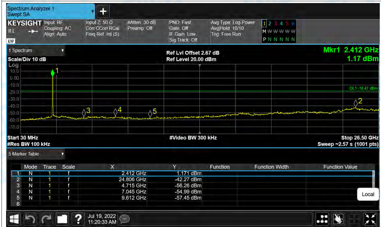
Tx. Spurious NVNT g 2412MHz Ant1 Emission
