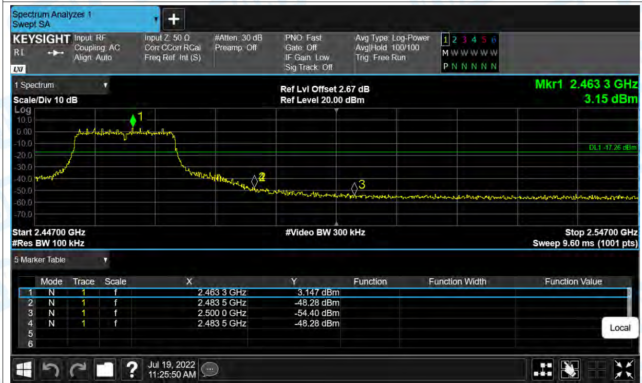
Band Edge NVNT g 2462MHz Ant1 Emission
