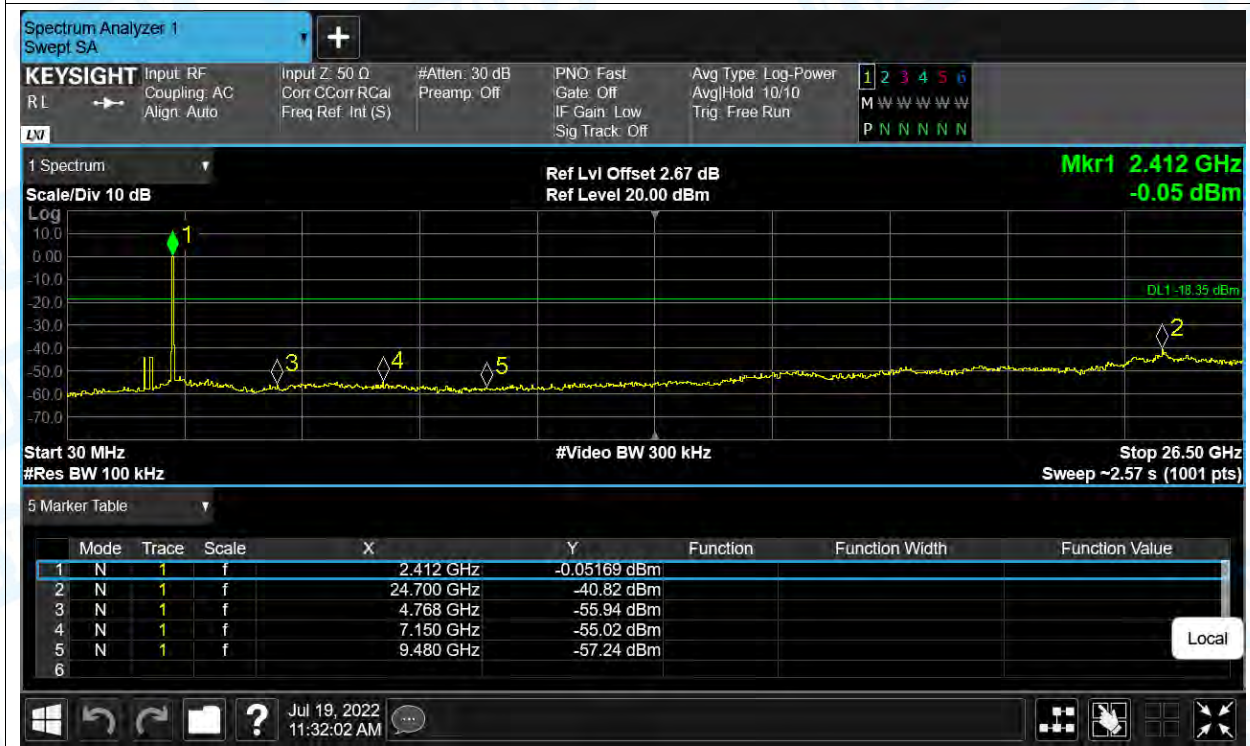
Tx. Spurious NVNT n(HT20) 2412MHz Ant1 Emission
