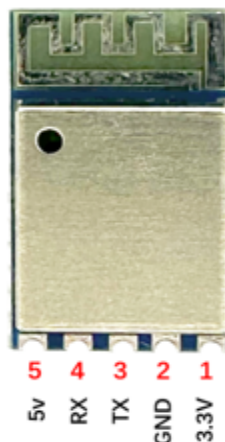
Figure 2. GY-BT2G Pin Definition Diagram
